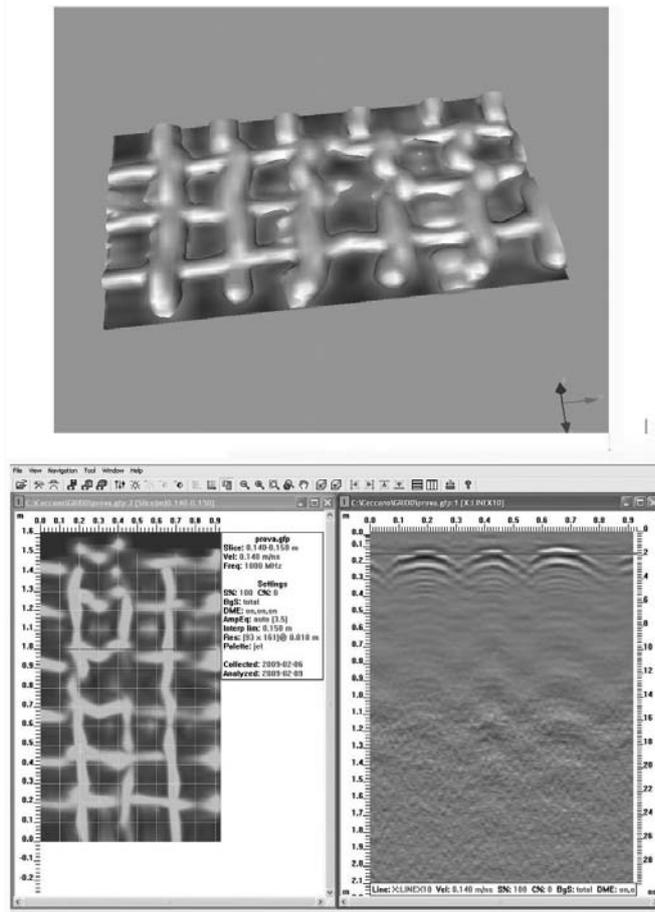
Figure 1: A typical GPR data processing: a 3D contour map, a pseudo-3D time slice and a radargram acquired on a concrete wall with reinforcing bars.
