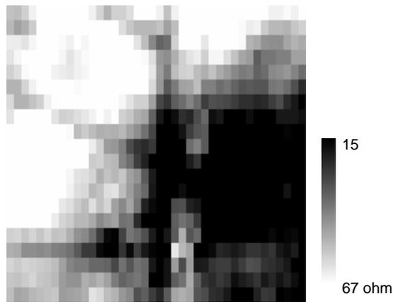
Figure 2: Showing a typical earth resistance data display of the seasonality test area from the 0.75m manual square array, values converted to apparent resistivity rho\_A (17.09.2009).
