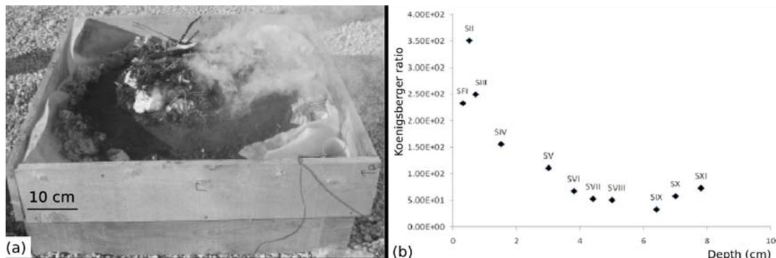
Figure 1: (a) experimental prehistoric hearth using soil of the Lazaret's cave (Nice, France); (b) vertical variation of the Koenigsberger ratio in the burnt soil of the experimental hearth. This diagram shows that remanent magnetization affects magnetic minerals close to the surface up to 1-2cm in depth.
