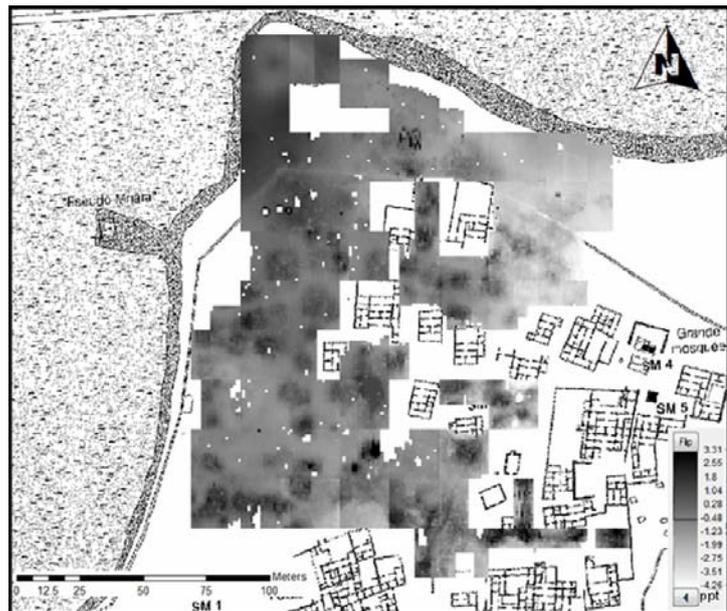
Figure 2: Magnetic susceptibility results from the electromagnetic survey (EM38B) at Songo Mnara (after Pradines 2005).
