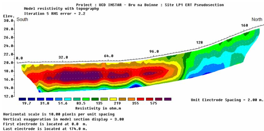
In order to investigate the sediments and the sub-surface structure of LP1 an N-S ERT transect was carried out using a Wenner array with 2m electrode or 'a' spacing. The modelled pseudosection is given in Fig 4.
