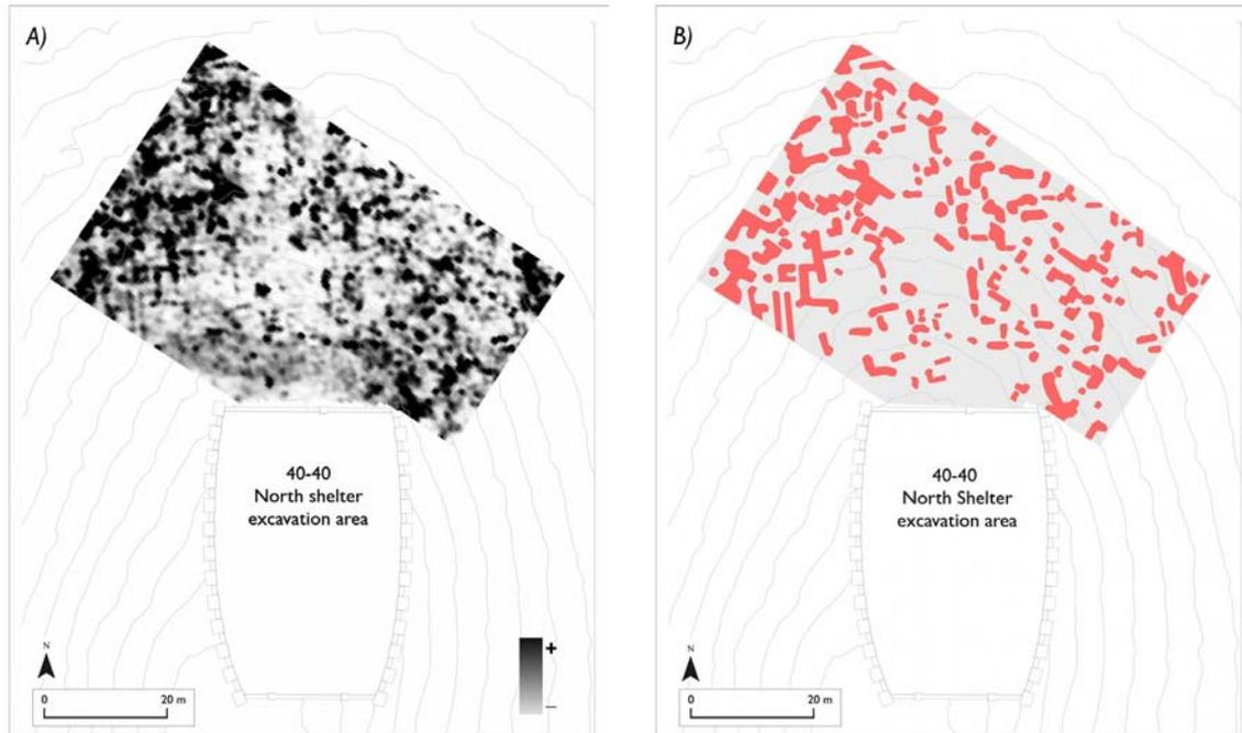
Results (A) and interpretations (B) of 500 MHz Ground-penetrating radar survey at Çatalhöyük in June 2010. Preliminary velocity analysis estimated this time slice at approximately 85cm below ground surface.
