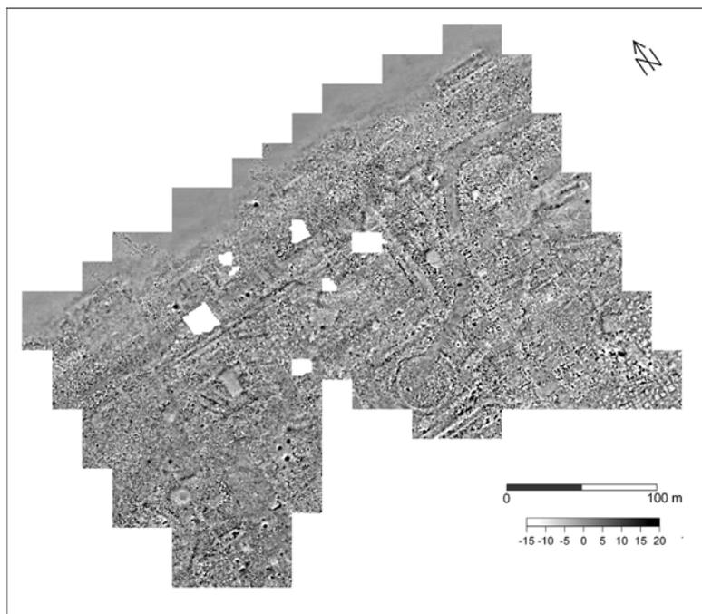
*Fig. 2: Magnetic map. Geoscan Research gradiometers FM256. Sampling grid 0.25 by 0.50m, interpolated to 0.25m by 0.25m. Low pass filter. Dynamics – 12/+17 nT (white/black).*
