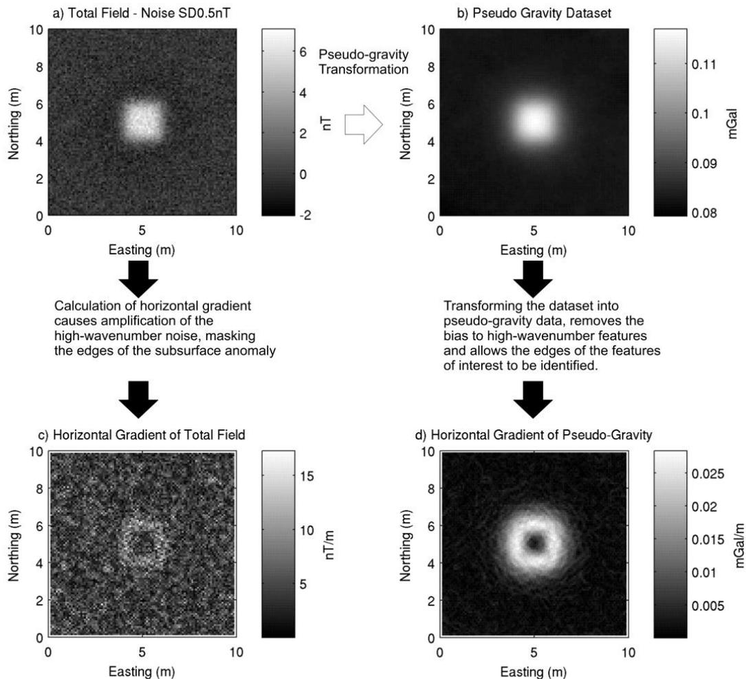
Figure 1: Total Field Data with 0.5nT SD Gaussian noise added; b) Pseudo-gravity dataset of (a); c) Total horizontal gradient of (a);. d) Total horizontal gradient of (b). Using the peaks in the horizontal gradient to identify the edges of the synthetic prism has been more successful here when applied to the data that was transformed to pseudo-gravity prior to the calculation of the derivative.
