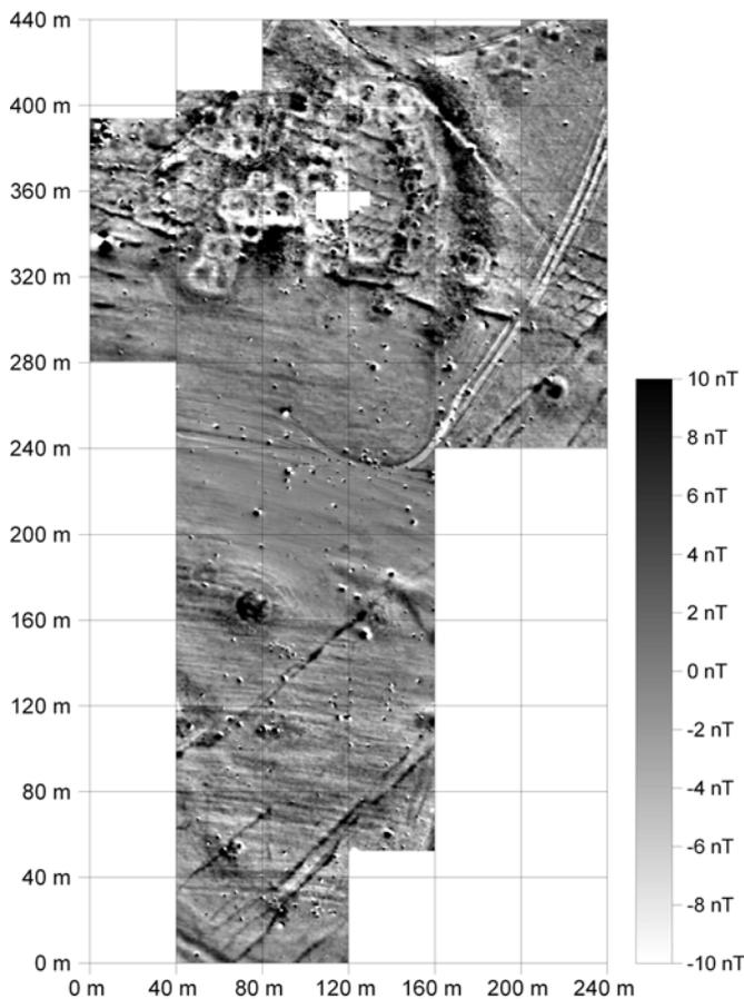
Fig. 2: Magnetogramm of Kabardinka II. Smartmag SM4G special in duo-sensor configuration, total Earth's magnetic field ca. 49.450 nT, dynamics +/- 10,00 nT in 256 grey values from black to white, grid size 40m x 40m, sampling density interpolated to 25cm x 25cm. In the upper part we see the layout of the houses in the shape of a horse shoe in the bottom we found single burials between the upstanding burial mounds.
