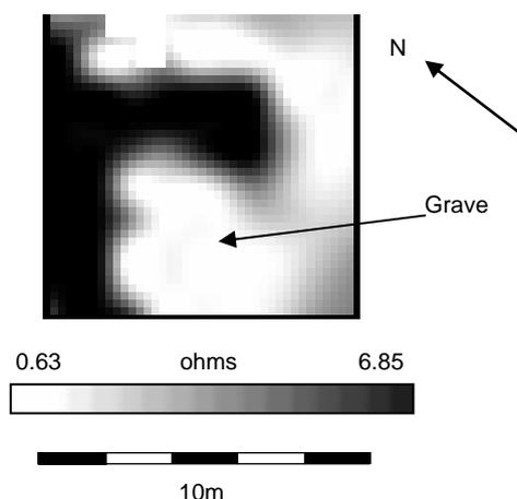
*Figure 1: Resistance survey showing greyscale image of enhanced data. Simulated grave shown as low resistance anomaly.*
