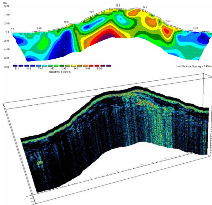
Figure 2: Preliminary Pole-pole electrical image (top) and 500MHz GPR (bottom) images revealing distinct inhomogeneity in the upper mound material. Electrical image created by a Tigre 64 and Res2Dinv. GPR image created by a Mala RAMAC X3M and GPR-Slice.
