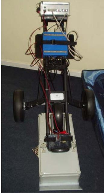
Our multi-channel Groundvue 3 is the fastest available, having simultaneously triggered antennas without cross channel interference. Data collection speeds in multi-channel mode or when using GPS/Total station are equivalent to 1000scans/sec with all channels operational. Simultaneous triggering also allows automatic depth calibration during survey. Groundvue GPRs comply fully with current European legislation.
