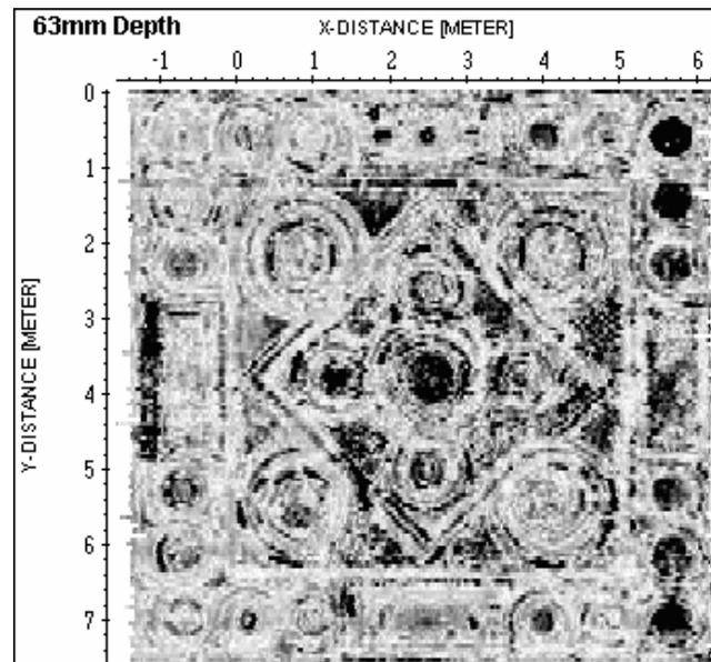
Figure 1: Time Slice from 4GHz GPR Survey of Cosmati Pavement
