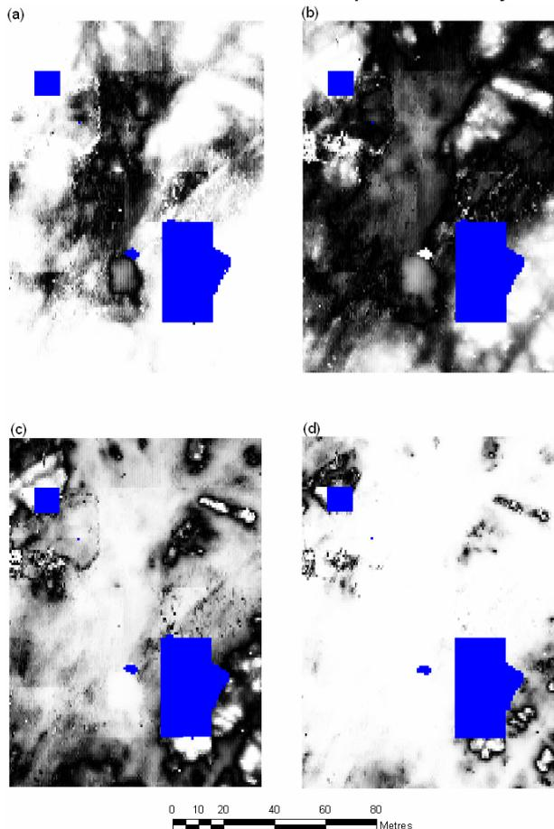
Figure 1: Estimated probability plots from the Hamar earth resistance data set with  $\beta_{k,l}=0$  for (a)  $k1=\log(R)=1.75$ , (b)  $k2=\log(R)=1.89$ , (c)  $k3=\log(R)=1.91$  and (d)  $k4=\log(R)=2.15$  where white is 0 and black is 1. For (a) please note the three linear features towards the left of the plot and in (c) notice the three anomalies, which would have fitted in between where three previous anomalies would have been.
