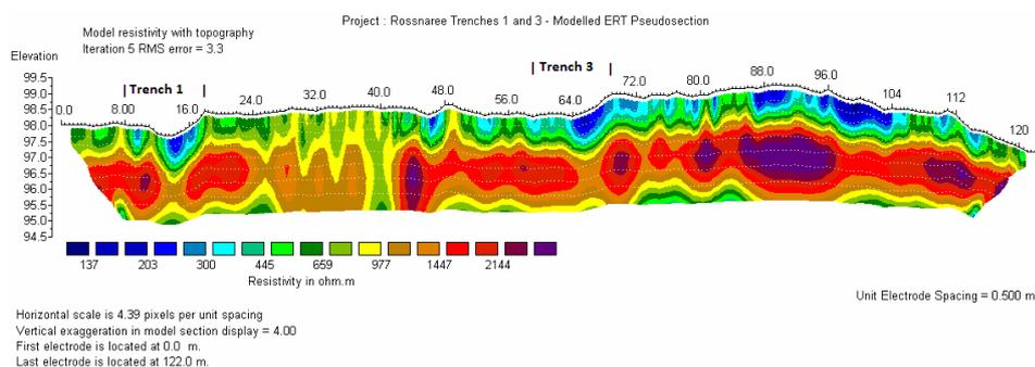
*Fig 3: ERT 7 – Modelled electrical resistivity tomography pseudosection (arbitrary height datum) with the location of Trenches 1 & 3 (vertical exaggeration x 4).*
