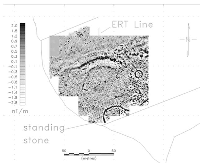
Fig 3: Preliminary Magnetic Gradiometry Results with Location of the Electrical Resistivity Tomography (ERT) Line
