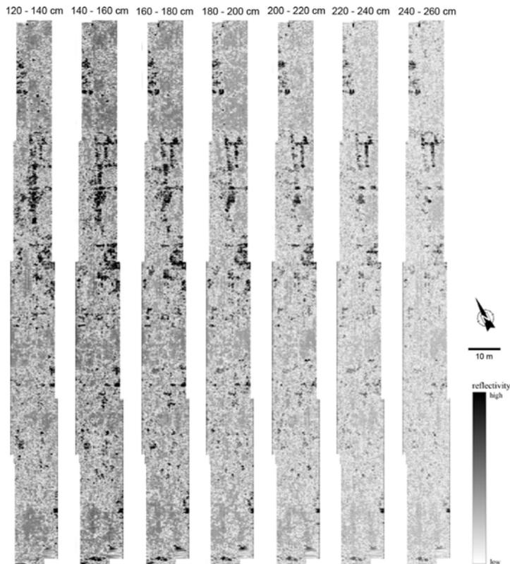
Fig. 2: Selection of depth slices with 20 cm thickness of Area 1 in Bustan el Khan. Grid size: 180 x 15m.
