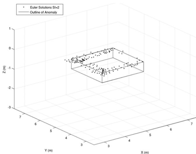
Figure 2: Euler deconvolution solutions for a structural index of 2. The solutions (circles) are clustered around the corners at mid-depth of the synthetic anomaly (solid lines).
