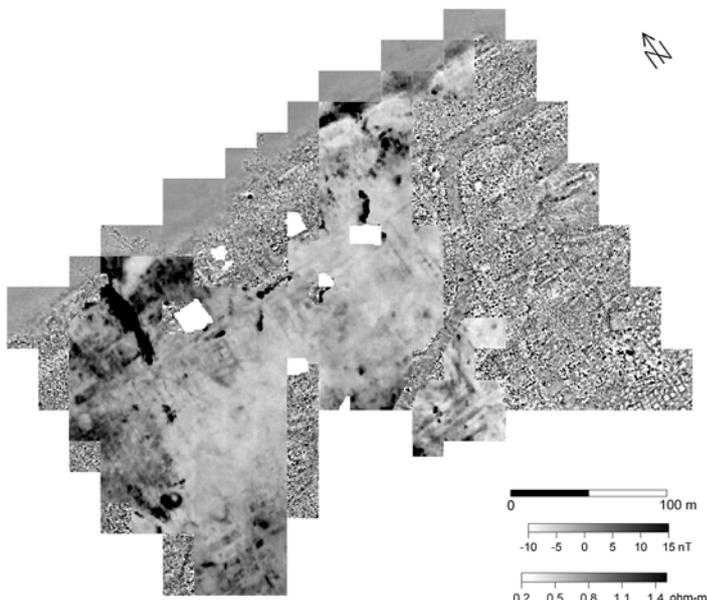
Fig. 3: Resistance map (superimposed on magnetic map). Geoscan Research resistivity meter RM15. Twin probe array, spacing of traversing probes 0.5m, remote probes 3.0m. Sampling grid 0.5 by 1m, interpolated to 0.5 by 0.5m. Low pass filter. Dynamics 0.25/1.5 ohm-m (white/black).
