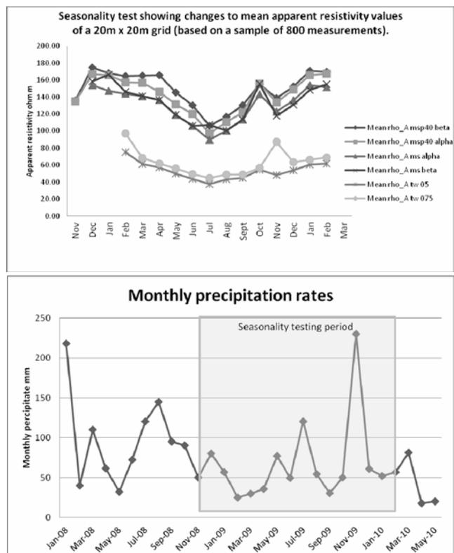
Figure 3: Showing the changing monthly apparent resistivity values of the 0.75m MSP40, 0.75m manual square, 0.5m and 0.75m twin probe arrays and the precipitation rate information from the local Met Office weather station.
