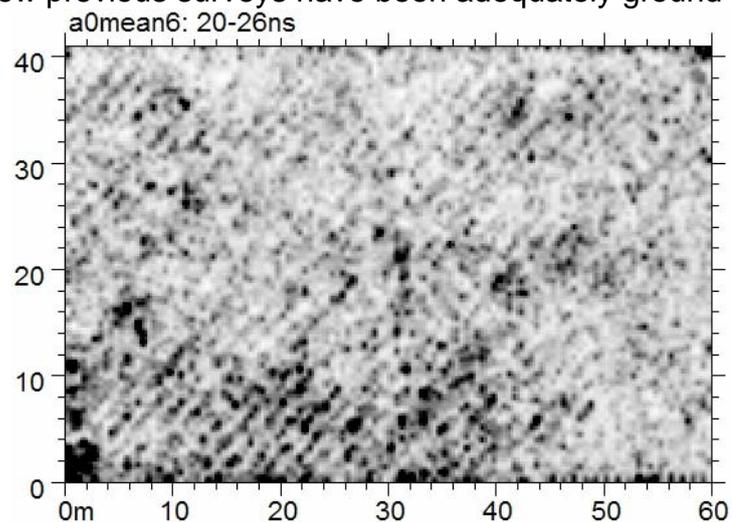
Figure 3: GPR Timeslice (20-26nS) from 250MHz survey at Flag Fen showing previous land use (either cultivation or peat workings) not visible from the surface features and on a different alignment to the recorded field system. Darker colours represent higher amplitudes, scales are in metres.
