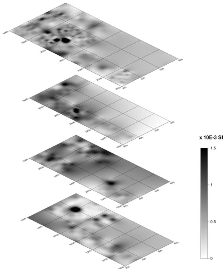
*Fig. 1: Susceptibility prospecting at the archaeological site Serteya a on three different layers (25 cm, 35cm, 45 cm, 65 cm from top to bottom) of the excavation. Magnetic susceptibility meter SM-30 (ZHinstruments, Czech Republic, sensitivity  $\pm 10E-7$  SI units, operating frequency 8 kHz), sampling interval 20 x 20 cm.*
