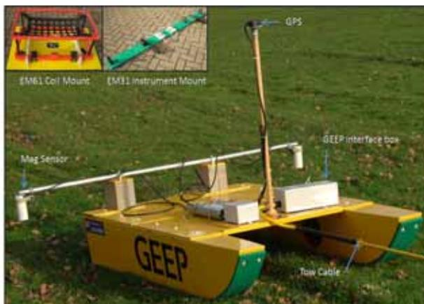
**Towed Instrument system;** Unique to Geomatrix is the Geophysical Equipment Exploration Platform (GEEP). GEEP offers the ability to record multiple data sets from complimentary instrumentation on a single towed platform. GEEP permits large areas to be surveyed in great detail and at high speeds whilst maintaining high data quality.
