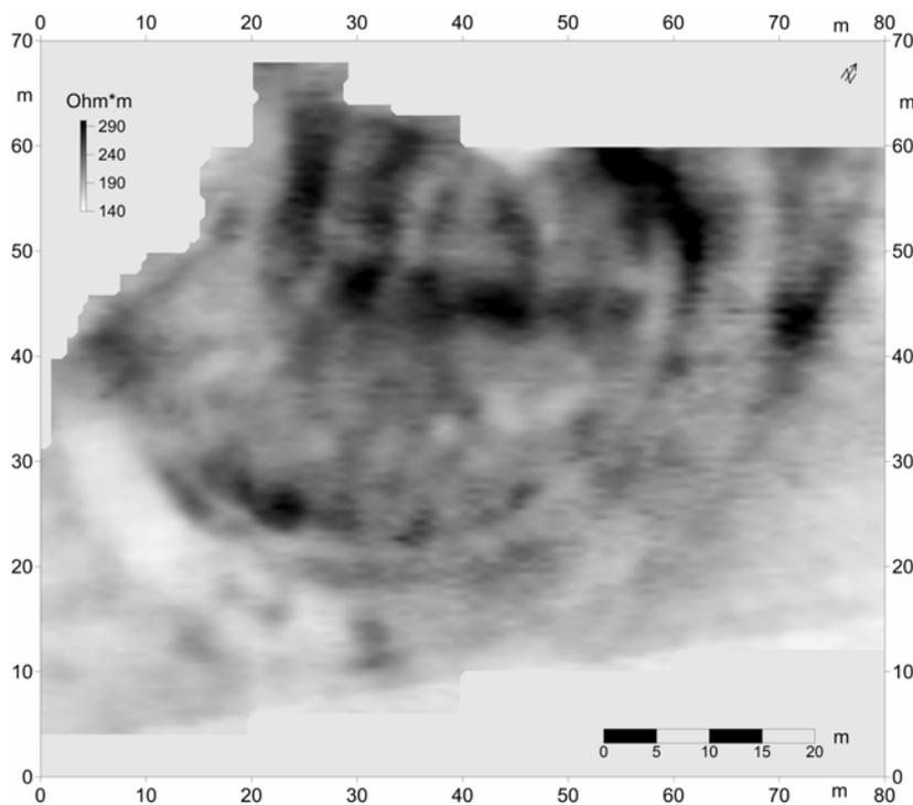
Fig. 3. Castle Wahrenholz. Apparent unfiltered resistivity map. Area 0.4 ha, RM-15, Geoscan Research, England, MPX15, parallel twin, point distance 0.5m by 0.5m.
