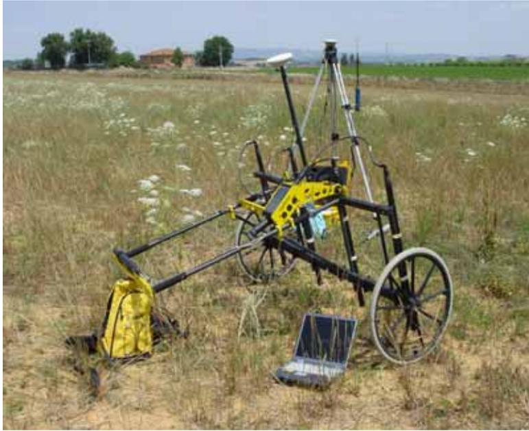
The data recording is carried out as a raster scan, with a length, width spacing and data point distance being set by the operator. The Magnetic data together with the X/Y (plus GPS data if used) position within the field is stored on an internal flash memory for later download.
