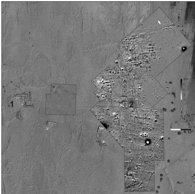
Fig. 2. Magnetic map of the western part of the site superimposed on a Google Earthpicture. 1 – Roman-age temple; 2 – platform of ashrine(?), Roman period. Measurements by T. Herbich and D. Święch; dataprocessing by T. Herbich. Fluxgategradiometers Geoscan Resaerch FM256, sampling grid 0.25 x 0.50m interpolated to 0.25 x 0.25 m; parallel mode, low pass filter.
