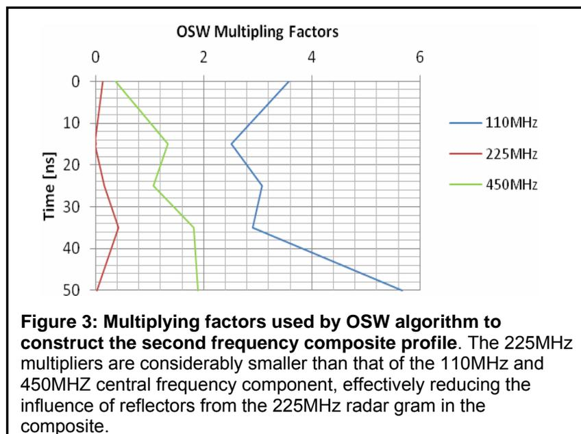
**Figure 3: Multiplying factors used by OSW algorithm to construct the second frequency composite profile.** The 225MHz multipliers are considerably smaller than that of the 110MHz and 450MHz central frequency component, effectively reducing the influence of reflectors from the 225MHz radar gram in the composite.
