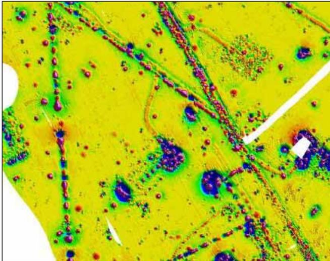
Figure 2: Magnetic results showing former structures and areas of concern on a former MoD site.
