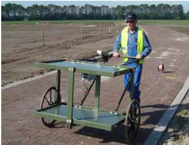
Based in Germany, SENSYS is specialized in the development and production of non-invasive geomagnetic and electromagnetic survey systems for various applications like rural and urban archaeological prospection. The product range varies from handheld magnetometer devices with one to five probes to vehicle towed multi channel systems with up to 32 magnetometer probes. These systems allow for detection in depths up to 3.5 to 4 m.
