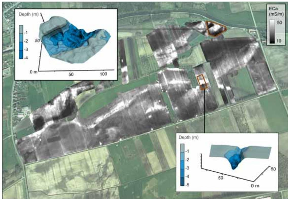
Figure 2: ECa data representative for a soil depth down to 1.5 m below the surface and orthophotograph of the survey area. The insets show outtakes from the palaeotopographical model.
