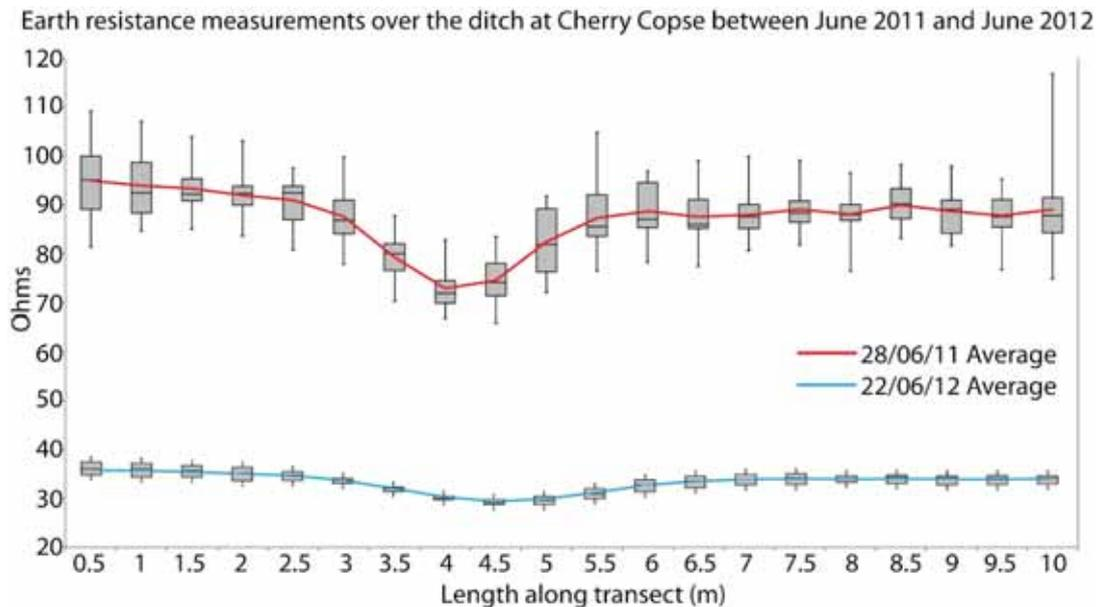
Fig. 3 Graph showing the differing earth resistance response caused by the ditch at Cherry Copse over the same area at different times of the year
