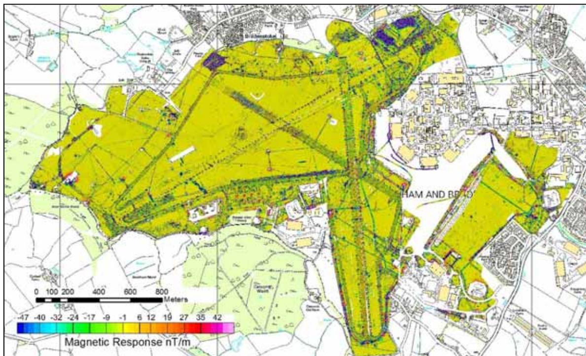
Figure 4: Magnetometer results from RAF Lyneham, acquired using a towed magnetometer array using 0.5m spaced foerster gradiometer probes under RTK GPS control.
