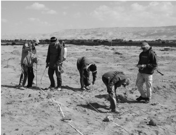
Fig. 4. Resistivity survey. On the left a team making and watering holes in the ground.
