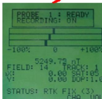
compensate disturbing influences from large anomalies at large distance to probe. Small magnetic anomalies close to the probe/surface will be displayed with high special resolution and high contrast.
