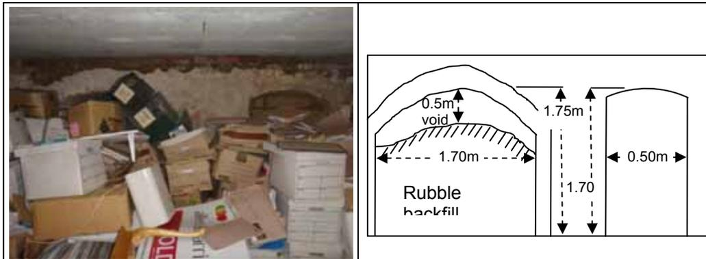
Figure 1: **Schematic diagram of the dimensions of the tunnels/ cavities emanating from number 40a High Street.** The tunnel depicted to the right of the diagram (Northern structure) is brick lined and it is possible to see into the air pocket. Whilst the narrower entrance (south structure) looks to be cut into the limestone bedrock but this is highly speculative due to the entrance being sealed. (Diagram not to scale)
