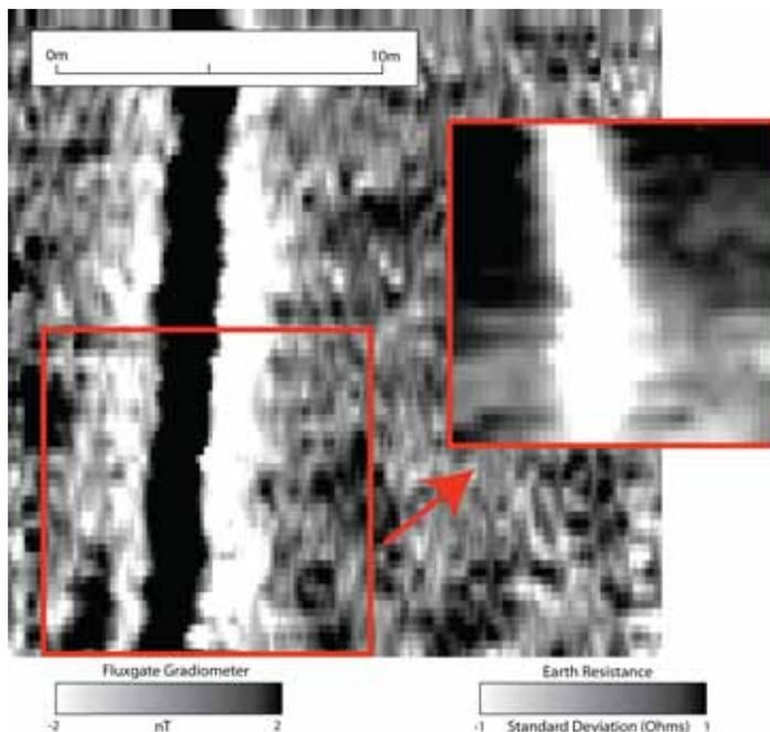
Fig. 2 Fluxgate gradiometer survey over the ditch at Cherry Copse with associated earth resistance survey area outlined in red
