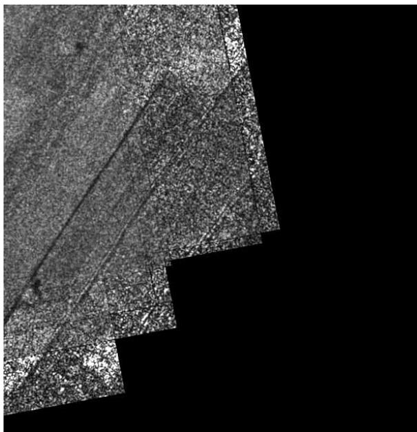
Fig. 2: Improvement of the signal/noise-ratio by stacking nine distinct SAR images. The effect can be shown very clearly at the edge of the composite image.
