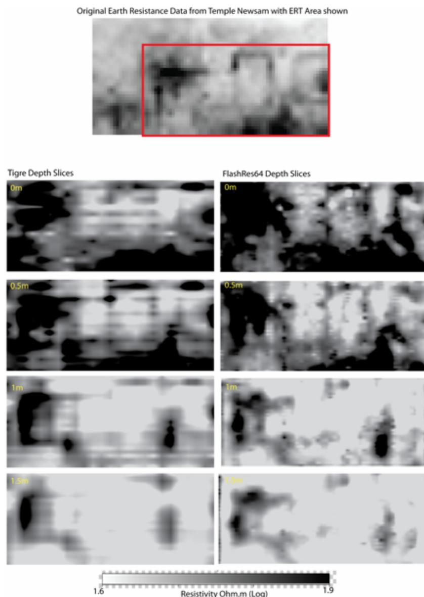
Figure 2. Comparative depth slices from semi fully-3D surveys using the Allied Associates Tigre ERI system and the FlashRes64. (Top) the semi-fully 3D survey area imposed on the earth resistance dataset; (Below, left) the Tigre ERI depth slices; (Below, right) the FlashRes64 ERI system depth slices
