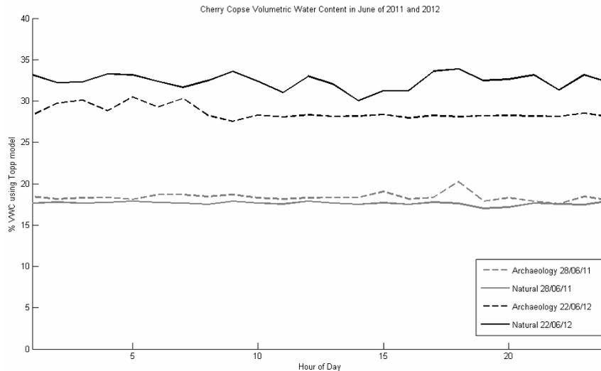
Fig.4 Calculated volumetric moisture content throughout each survey day from two TDR probes placed at depths between 20-30 cm within the ditch-fill and the 'natural' at Cherry Copse
