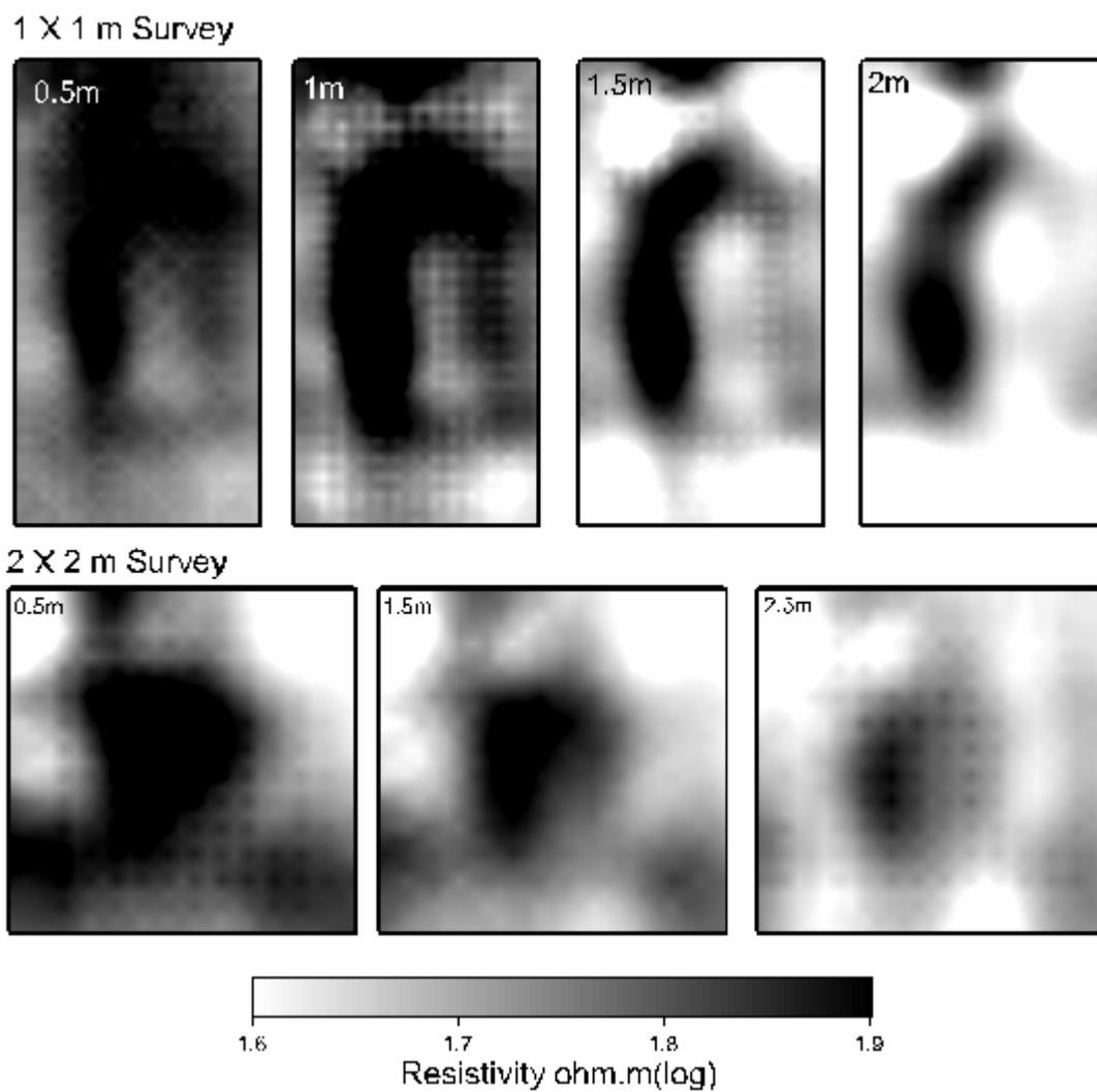
Figure 4. Data collected from a full-3D survey over the rectangular building at both 1m gridded probe separation, and at 2m gridded probe separation.
