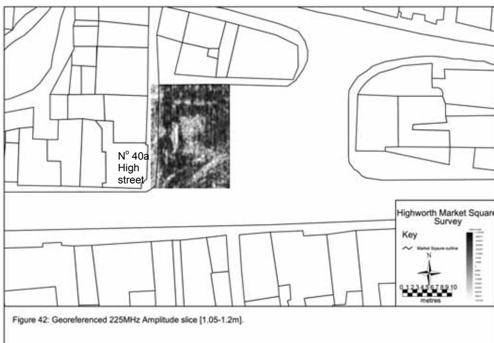
Figure 42: Georeferenced 225MHz Amplitude slice [1.05-1.2m].
