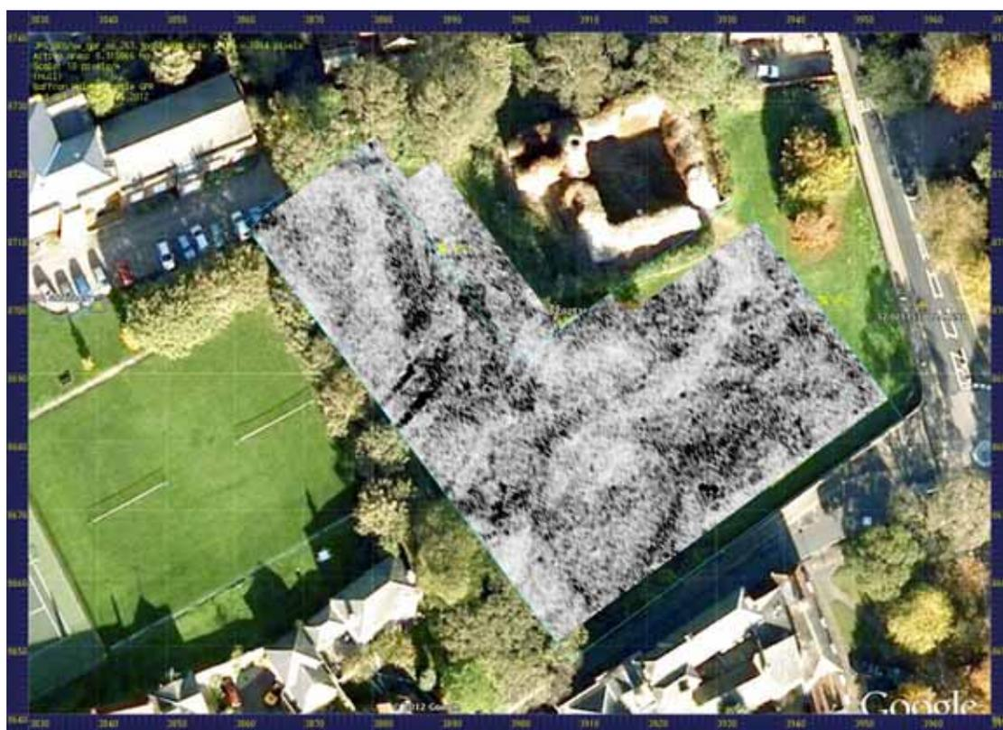
**Figure 2. GPR timeslice (Mala 500 MHz instrument) at 34 ns ( $\approx 1.7\text{m}$ ).**
