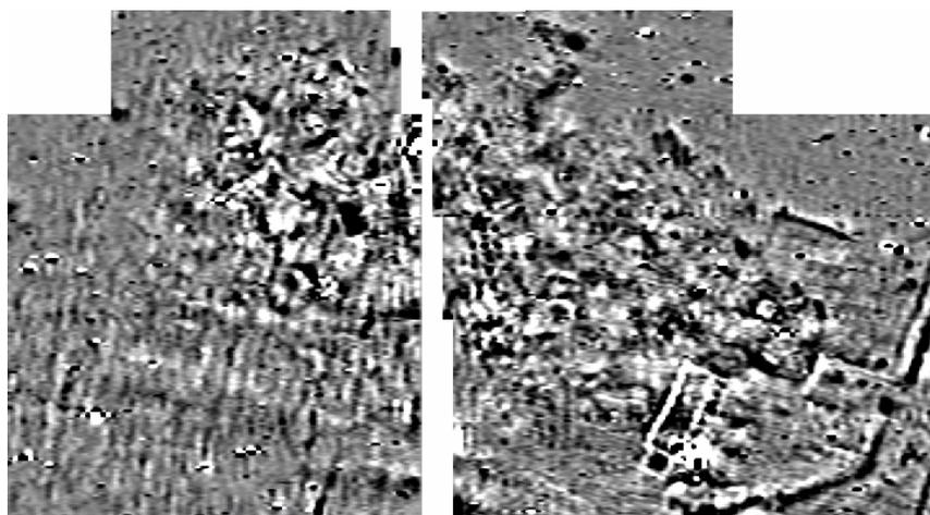
Figure 1. Fluxgate gradiometry results from a multi-period intensively occupied settlement undiscovered by other methods adjacent to the site of a 'mirror' burial. Note towards the bottom right of the plot the clear negative response of the walls of a Roman building, one wing of a range detailed further by earth resistivity. Interpolated 0.125x1.0m reading intervals. Grid size 20x20m. Survey area 160x100m. Black positive & white negative. Clipped at -5 to +5 nT
