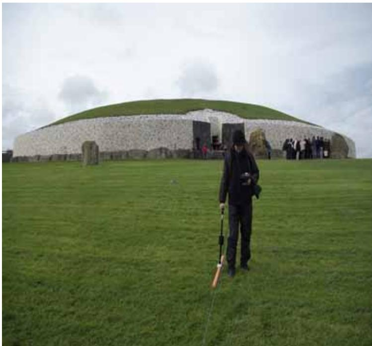
The MiniExplorer is designed for agriculture, forestry or archaeology applications providing detailed results at depths up to 1.8m. The instrument allows simultaneous measurement with 3 depth ranges (0.5, 1, & 1.8M) making this an ideal complement to the traditional surveying techniques. Lightweight, fast and GPS compatible this new product will offer increased knowledge of the subsurface. Sales or rental of the Mimi Explorer are available.
