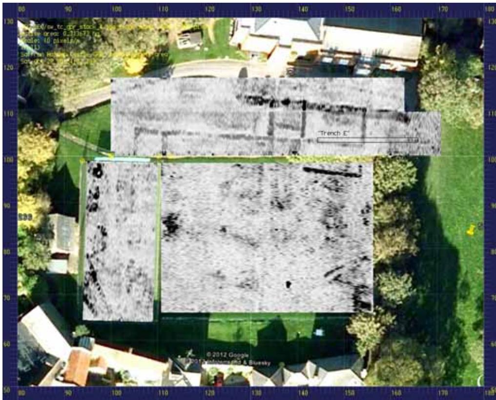
**Figures 4a (above) & b.** Composite GPR timeslices for the tennis courts area. Survey grid aligned to tennis courts north fence. Background image Google Earth. The location of 'Trench E' from the 1973 excavations is indicated.
