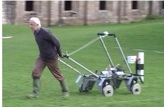
The platform comprises four spiked wheels set 0.75m apart on a rugged aluminium and stainless steel frame. A Geoscan Research ADVANCED RM85 Resistance Meter and Expansion Port Interface Box 1 are mounted centrally. Provision is made for attaching a towing system.
