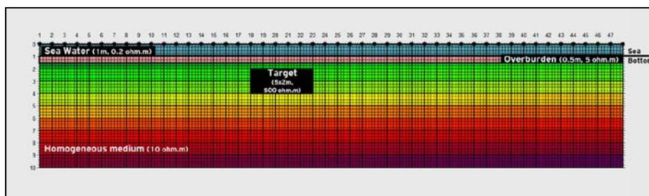
*Fig. 1 Synthetic model for ERT marine for shallow sea water measurements. A target ( $500\ \text{ohm}\cdot\text{m}$ ) is embedded in a homogeneous medium ( $10\ \text{ohm}\cdot\text{m}$ ),  $0.5\text{m}$  below an overburden layer ( $5\ \text{ohm}\cdot\text{m}$ ). Sea water column is set to  $0.5\ \text{m}$  (resistivity  $0.2\ \text{ohm}\cdot\text{m}$ ).*
