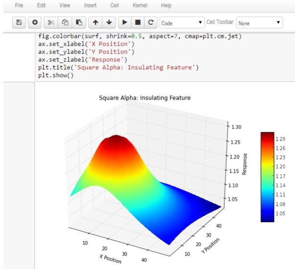
Fig. 2 Numerical modelling and display of resistivity responses over three-dimensional features.
