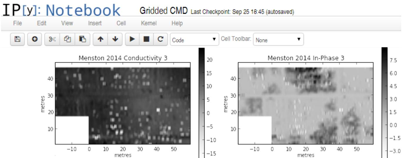
Fig. 1 Automated management and re-gridding of electromagnetic induction data, allowing an easy, streamlined importation into conventional data processing packages.
