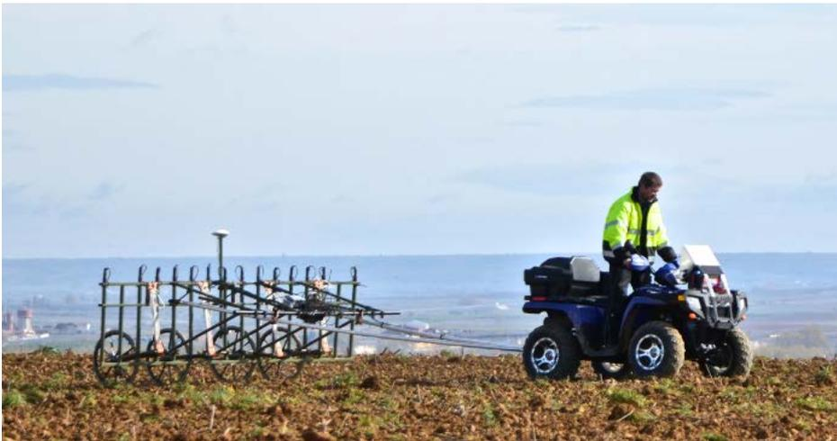
Fig. 2 Magneto MX V3 16-channel system with modular cart
