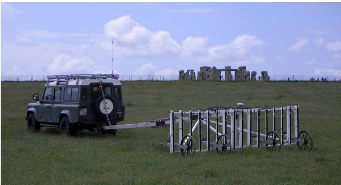
*Fig. 4 Magneto MX 16-channel system during a survey session at Stonehenge*
