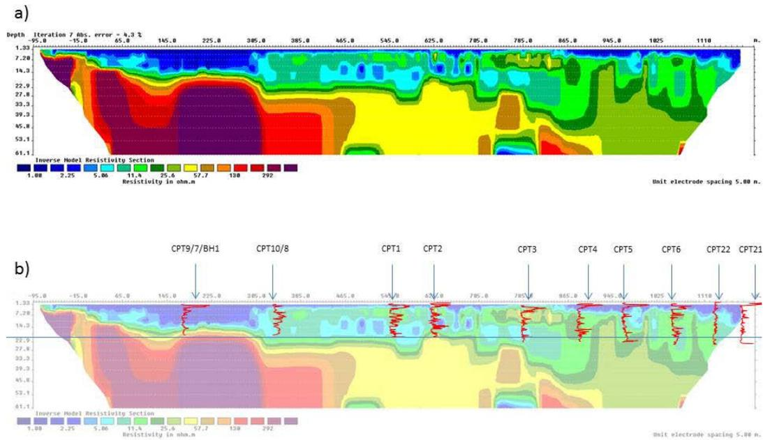
Fig. 3 West Street Selsey Channel, FDEM and ERT section
