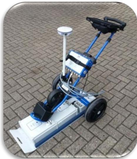
**Towed Instrument system;** unique to Geomatrix is the Geophysical Equipment Exploration Platform (GEEP). GEEP offers the ability to record multiple datasets from complimentary instrumentation on a single towed platform. GEEP permits large areas to be surveyed in great detail with multiple sensors whilst maintaining high data quality.
