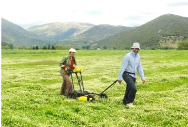
*Fig. 1 Noggin Smart Cart equipped with 250MHz antenna.*
