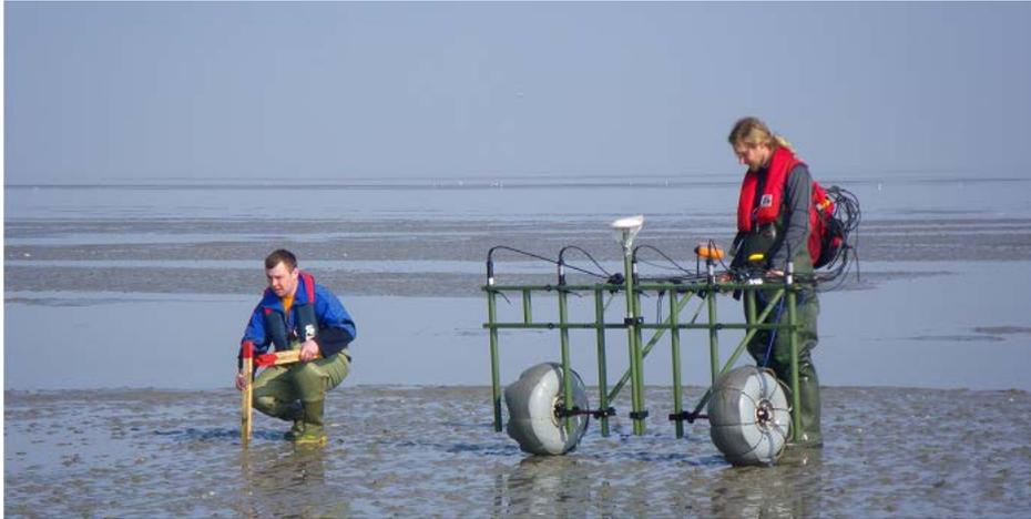
*Fig. 3 Magneto MXPDA 5-channel cart system during a survey session at the Wadden Sea with customized wheels*
