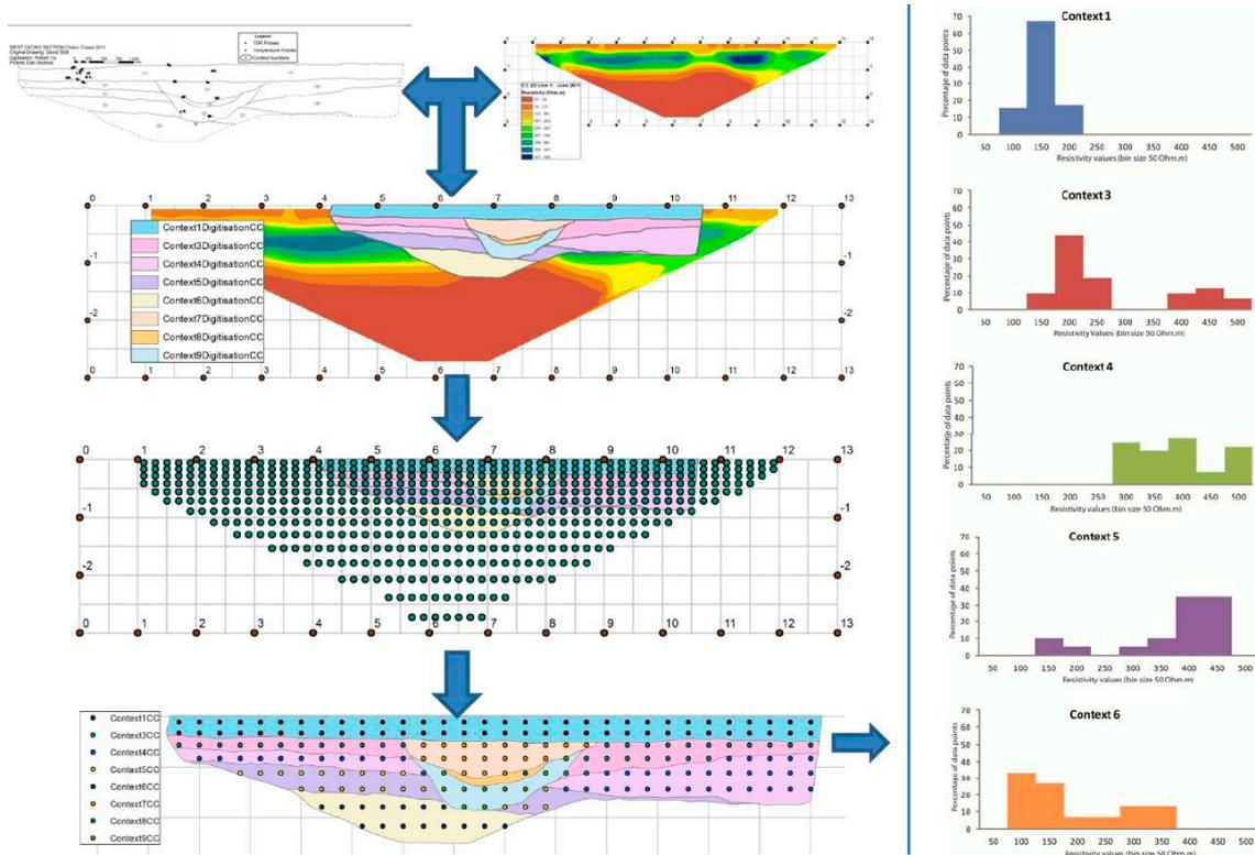
Fig. 1 Extraction of resistivity data from ERI profiles into separate archaeological contexts
