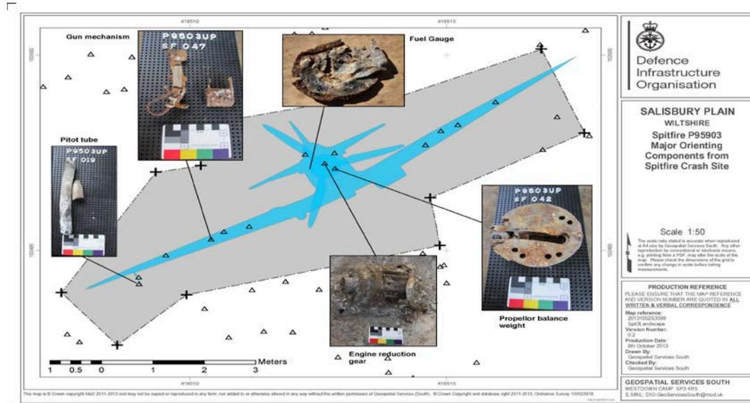
Fig. 2 Map of the Spitfire P95903 aircraft parts excavation
