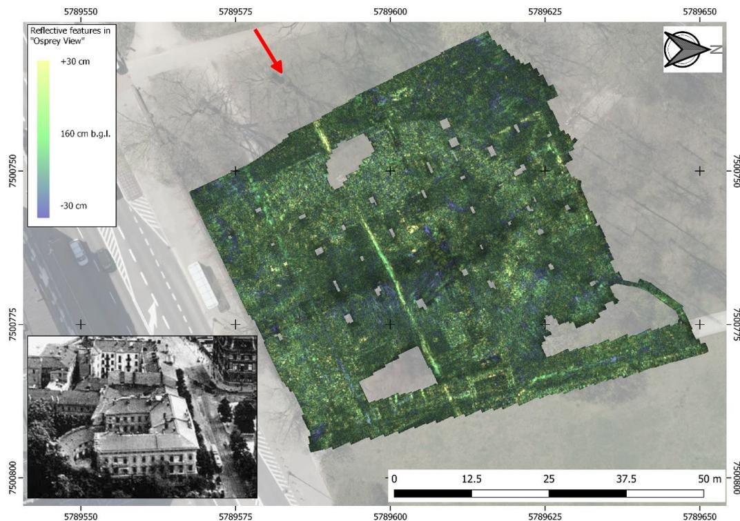
Figure 10: Calculated depth slice of the results from the Królewska tenement houses sector, presented in OspreyView visualisation with a central depth of 160 cm. In the bottom left a pre-war aerial picture of the houses is shown. The red arrow indicates the perspective of the picture.
