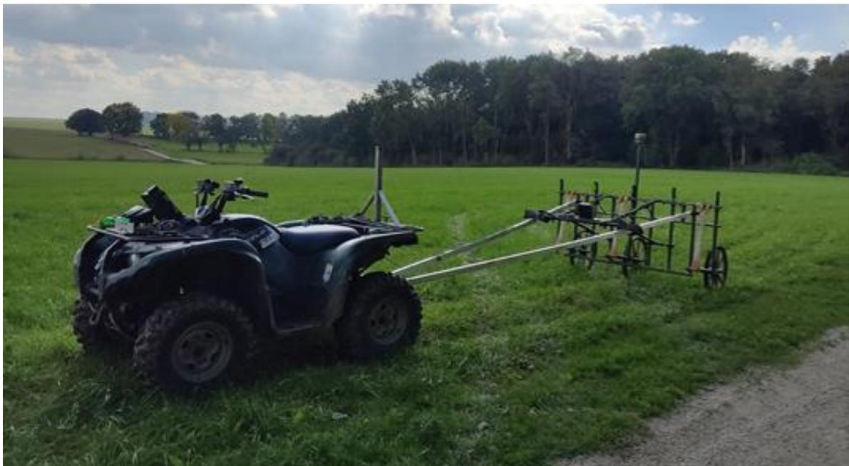
*Figure 5: Magnetometer survey near Hougoumont Farm, Waterloo.*
