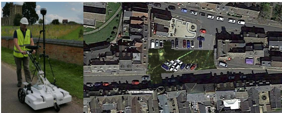
Fig 2. - The upper image shows the raptor cart 450MHz system (left) and a fully processed dataset generated in the condor software (Right). The results identify a number buried utilities as well as an infilled basement (the high amplitude rectangular response in the North East of the dataset) from a demolished commercial property. The property is present on a map of the market square dating from 1779.
