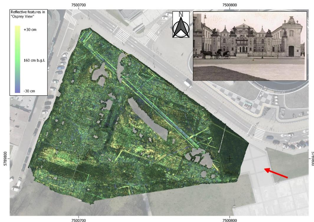
Figure 9: Calculated depth slice of the results from the Brühl's Palace sector, presented in OspreyView visualisation with a central depth of 110 cm. In the top right, a pre-war picture of the entrance gate to the palace is shown. The red arrow indicates the perspective of the picture.
