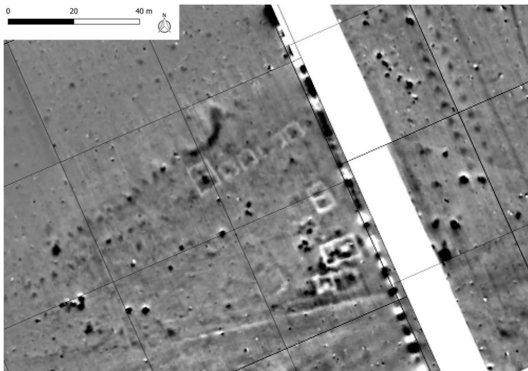
Figure 11: Section of the magnetogram in Ruffenhofen showing the relevant part with the Roman grave monuments. Scintrex SM 4G-Special Caesium Magnetometer, duo-sensor configuration, sensitivity:  $\pm 10$  pT, dynamics:  $\pm 10$  nT in 256 greyscales, sampling rate: 50 x 25, interpolated to 25 x 25 cm, 40-m-grid. Archive-No. Ruf00b.
