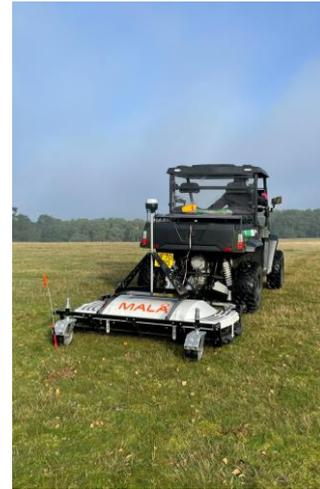
Figure 1: MALÅ MIRA HDR multichannel 3D GPR array
