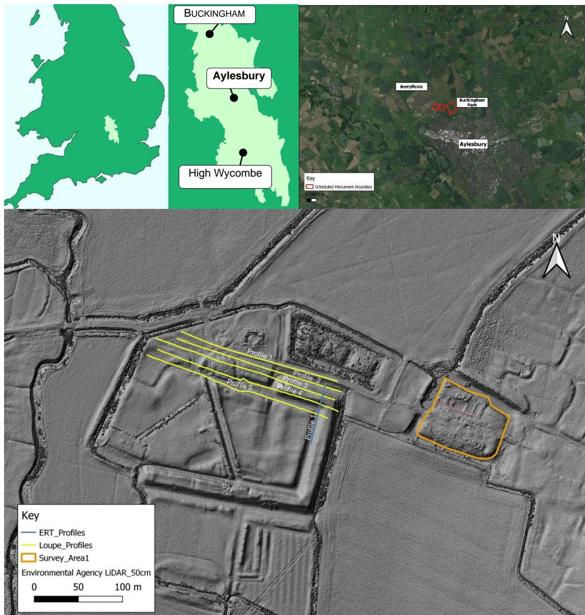
Figure 2: Survey Area 1 is where the Tudor Manor house is believed to be located. Five profiles were recorded with the Loupe TEM system over the earthworks forming the water gardens.
