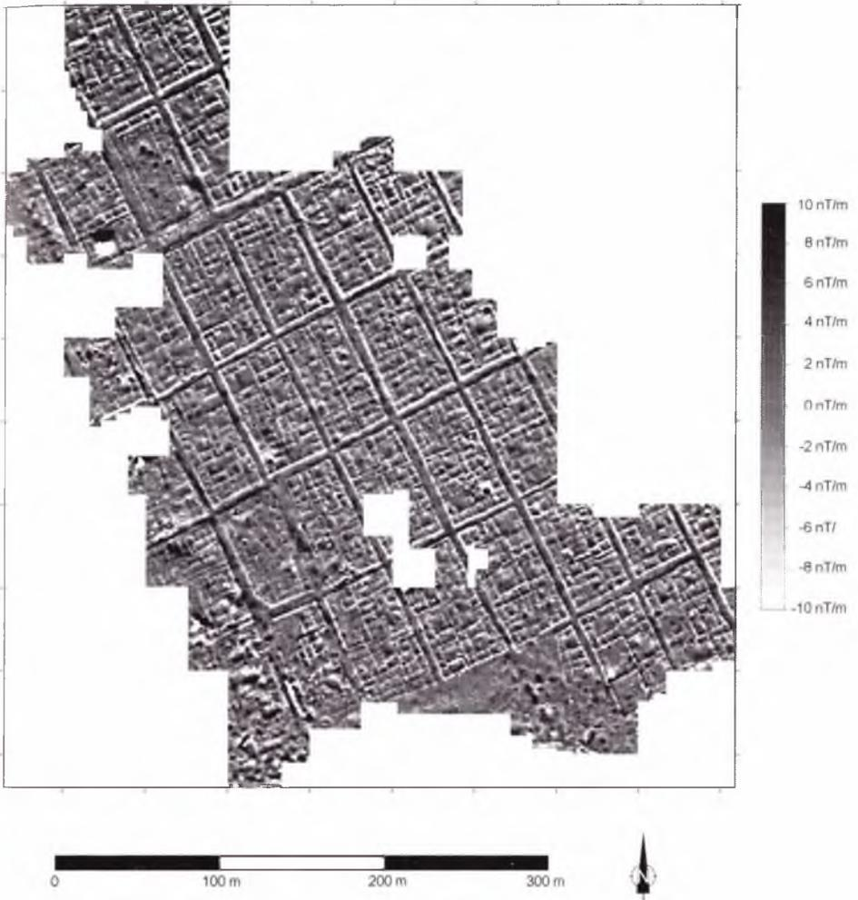
Fig. 3. Dura-Europos. Magnetic map. Caesium gradiometer (G858, Geometrics).
