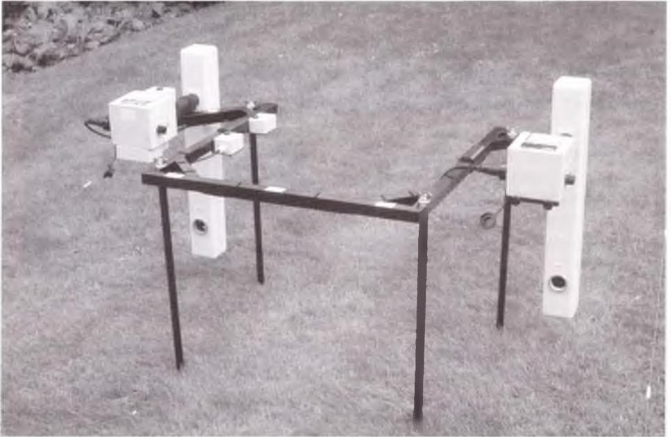
Fig. 2. Dual gradiometer system using an FM 256 (master) and FM 36 (slave) mounted on a CF6 carrying frame.
