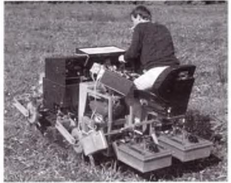
Fig. 1. Modified small caterpillar vehicle for simultaneous recording of GPR and resistivity data (spike wheels). Two antennas mounted with a distance of 50 cm at the end.
