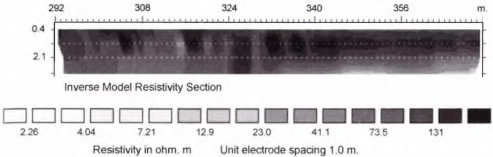
Fig. 2. Burgaz. Profile n 606, result of resistivity inversion.
