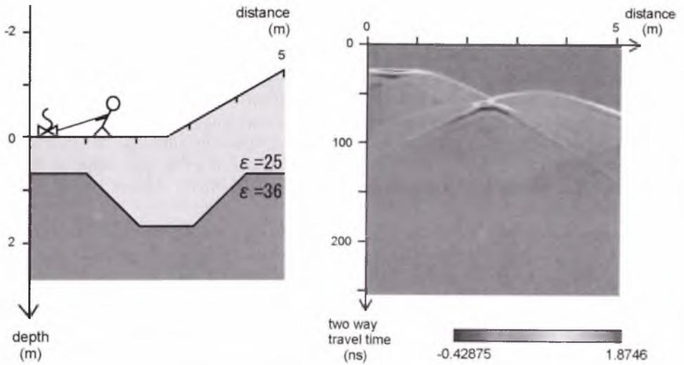
Fig. 1. (a) GPR simulation model, (b) simulated GPR image.
