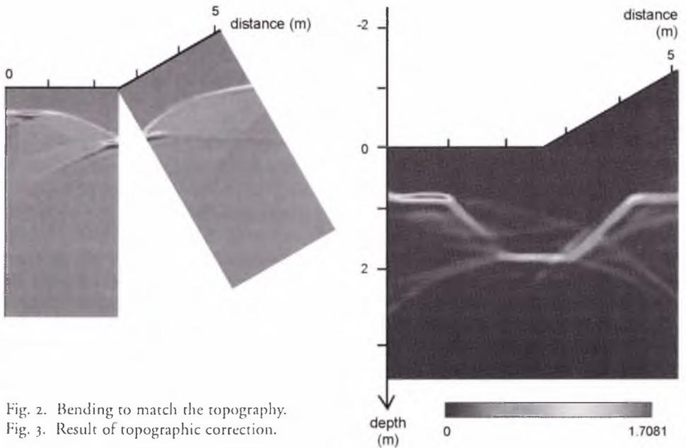
Fig. 2. Bending to match the topography.
