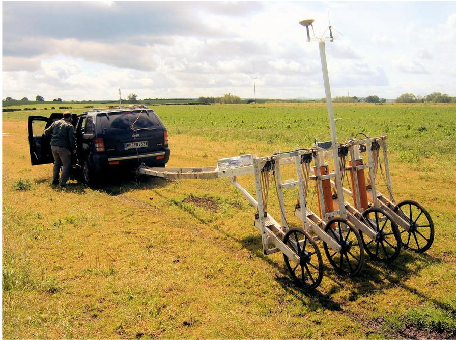
**Figure 5.** Squid system developed by Schultze and colleagues at the Institute for Physical High Technology, Jena (Germany).
