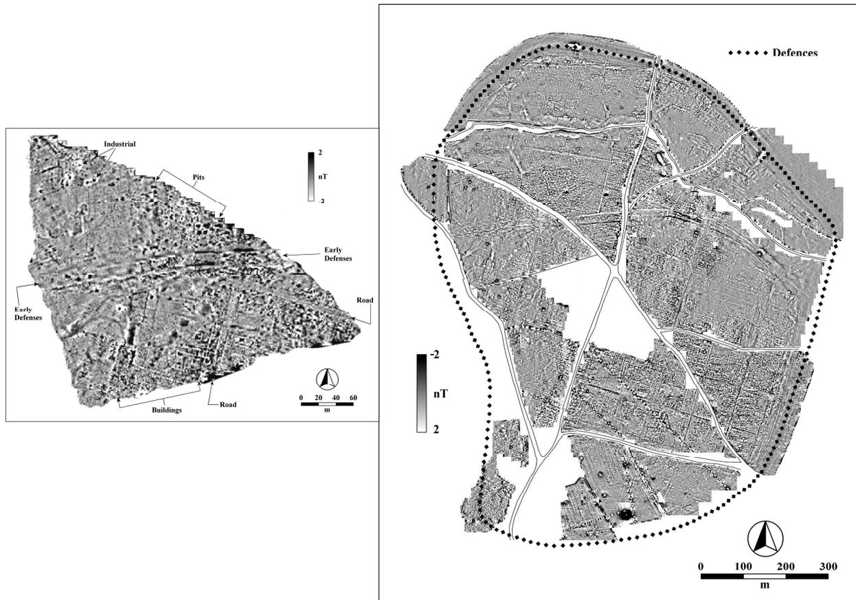
**Figure 14.** On the right hand side is an image of the magnetic data of the Roman City of Wroxeter collected by GSB Prospection and the AMLab using Geoscan Research FM series magnetometers. On the left hand side is detail from one of the areas. Note the change in vertical scales. The figure is after Gaffney and Gater 2003 and is courtesy of the two survey groups.
