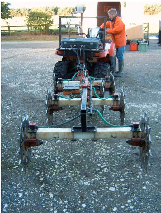
In addition to data collection at great speed the SQUID technology allows very accurate measurements, easily outperforming other magnetic devices (Schultze et al 2005). The latest incarnation of the French mechanised resistivity system also has its roots in a non-archaeological application (viculture) (**Figure 6**). Again, this is directed by real time GPS and can measure three depths of resistivity simultaneously (Dabas and Favard, 2004).
