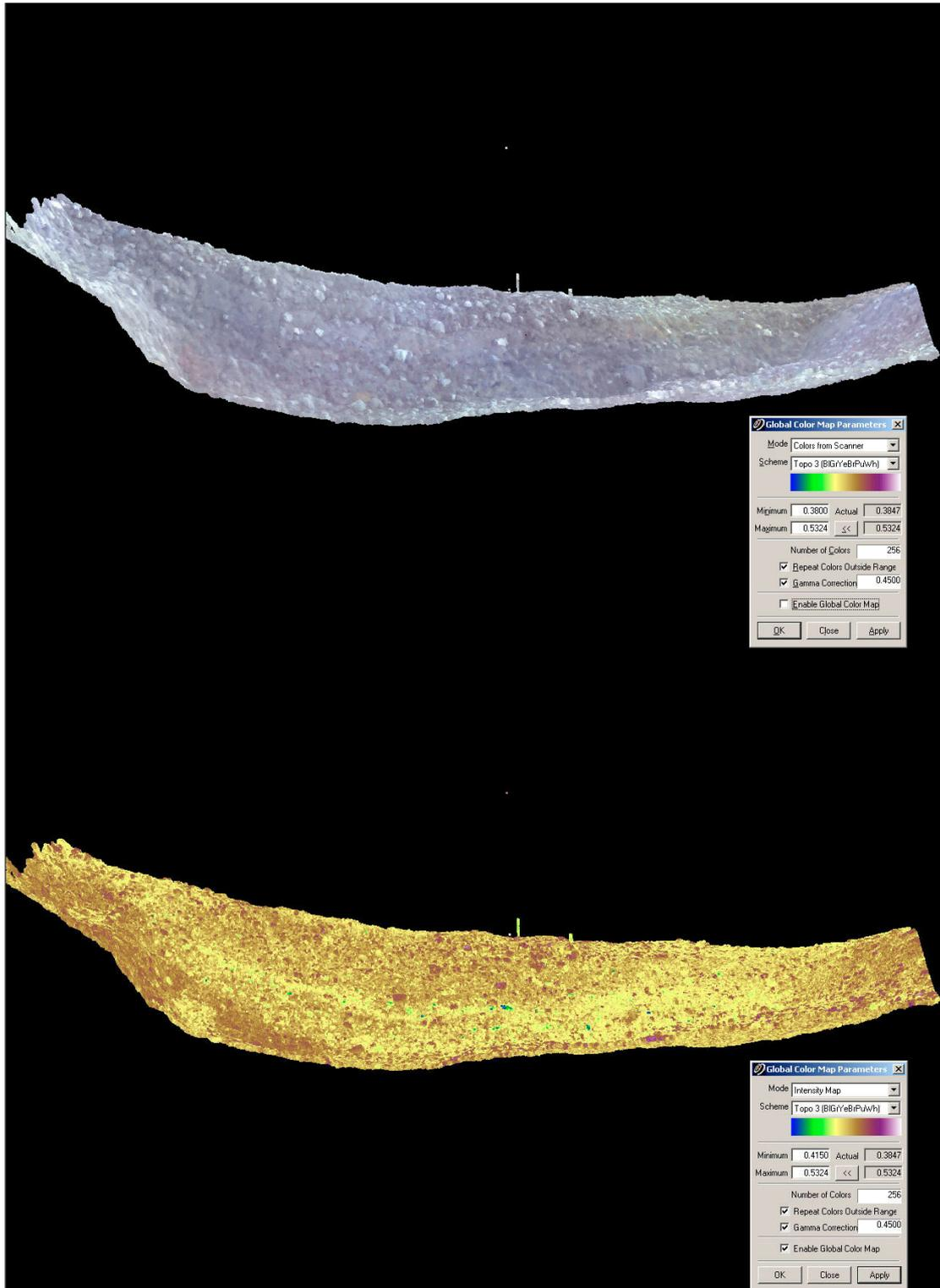
**Figure 9** Images of a cess pit profile scanned using a Leica Cyrax laser scanner. The top image shows the 3D data overlain with the photographic image of the pit, the bottom shows laser intensity data and illustrates the different stratigraphic information potentially provided by laser intensity mapping (source Professor Mike Fulford).
