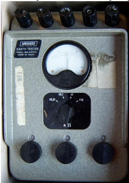
The first surveys involved unwieldy apparatus culled directly from what we now call Earth Science; this included basic measurement devices such as the Megger Earth Tester (**Figure 1**) and the classic resistivity arrays such as the Wenner. Processing power to manipulate the data was also minimal.
