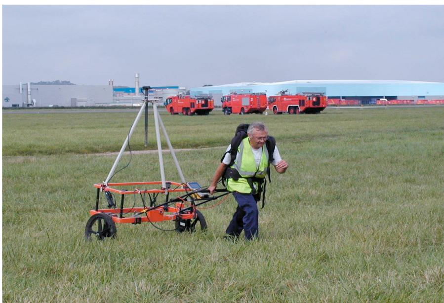
**Figure 3.** Ian Wilkins of GSB Propection Ltd using an EM-61 with dGPS. Photograph courtesy of GSB.
