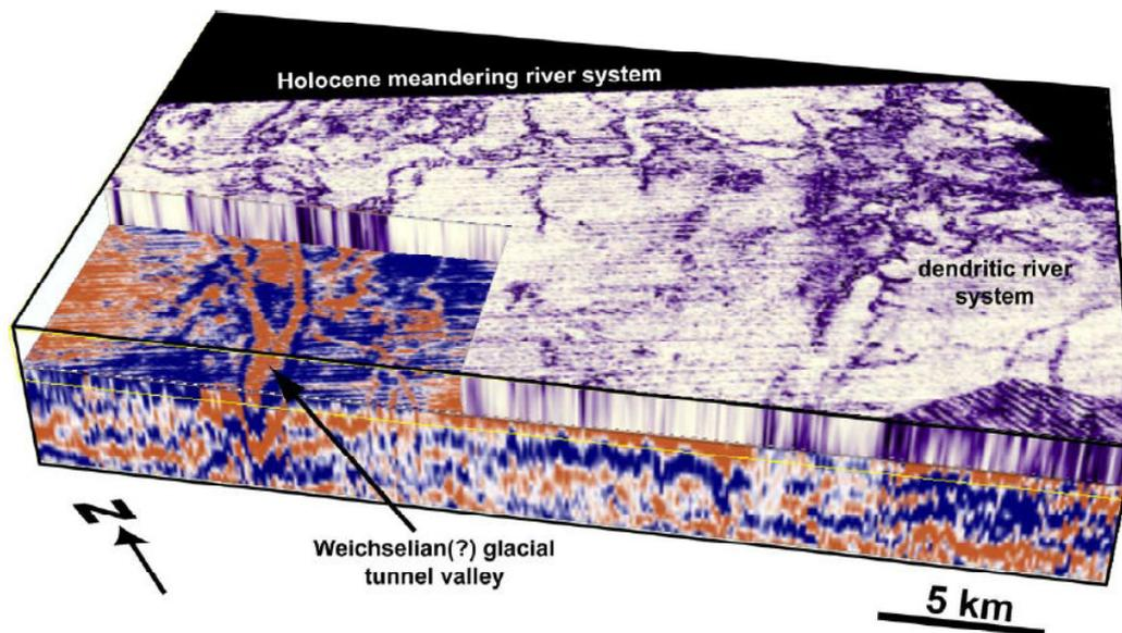
**Figure 12.** Seismic amplitude volume overlain by a seismic coherence volume. The figure demonstrates that the probable Weichselian tunnel valley pre-dates the meandering river system which is consequently of Holocene age (after Fitch et al. 2005).
