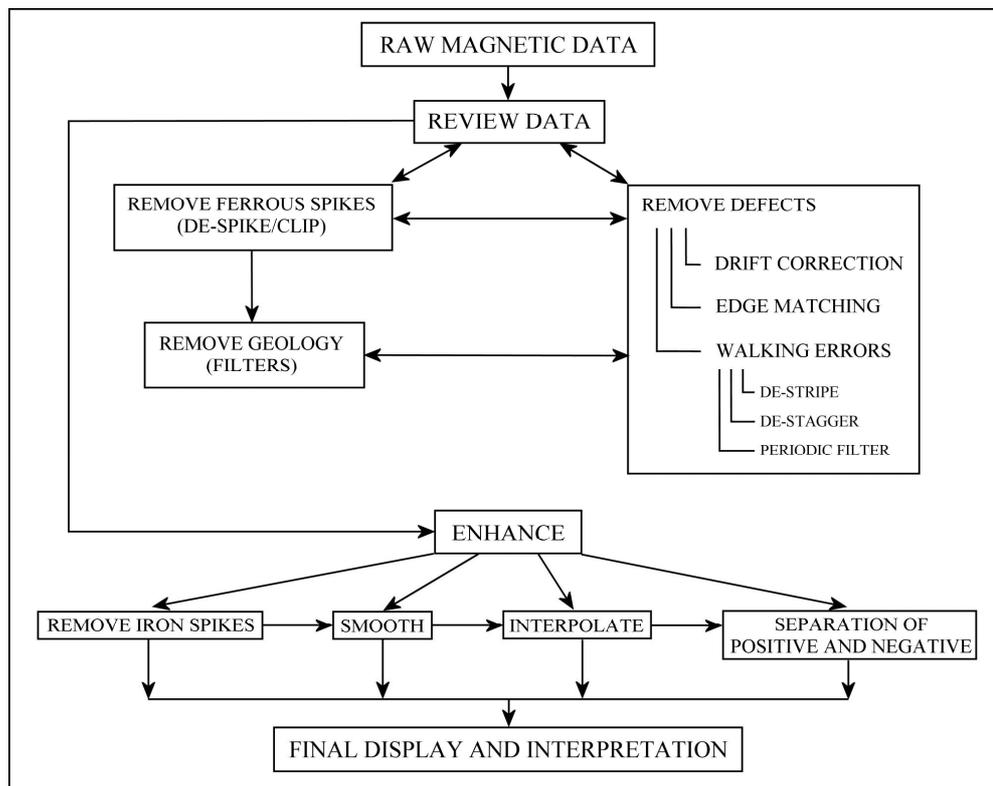
**Figure 10.** Typical flow chart for processing magnetometer data. From Gaffney and Gater 2003.
