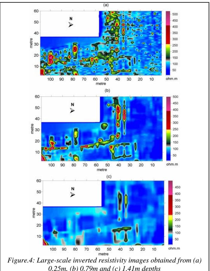
Figure 4: Large-scale inverted resistivity images obtained from (a) 0.25m, (b) 0.79m and (c) 1.41m depths
