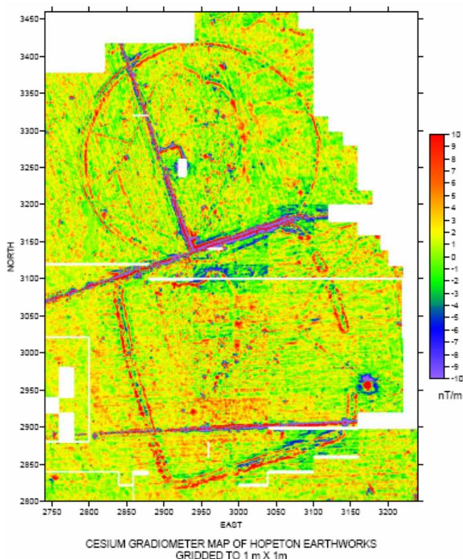
lines marking the earthwork wall lines are separated by about 10 to 15 m and the magnetic maxima are 15 to 20 nT above the background. The anomalous streaks that occur at various places are caused by deep plough scars.
