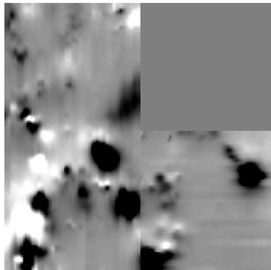
*Fig. 3: Sternwartgelände München Bogenhausen: Magnetogram of the first geomagnetic observatory. The strong anomaly on the right side of the picture is in a great depth and is exactly inside the south tunnel of the substructure of the geomagnetic observatory.*
