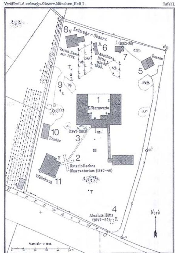
Fig. 2: Sketch of the area from 1904. (1) Main building of the Sternwarte; (2) first geomagnetic observatory 1840-1846; (3-4, 6-8) other observatories for geomagnetism of later times; (9) "Earthquake house"; (10) Remise; (11) residential house.
