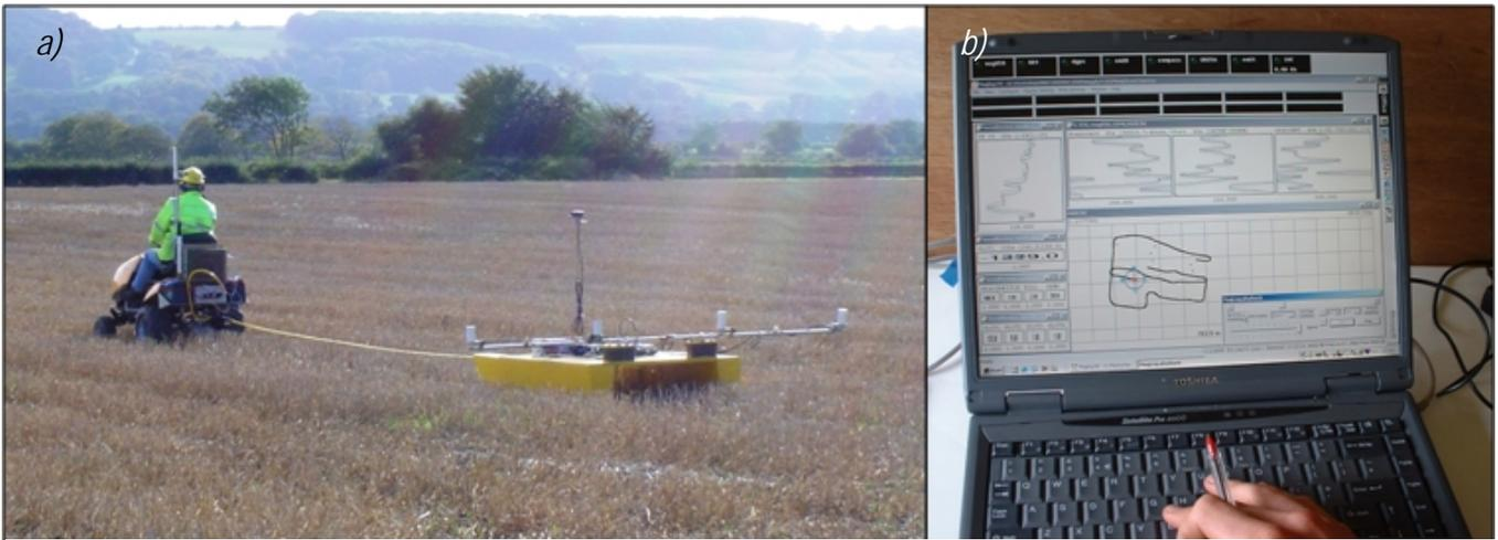
Figure 1: The two components of the Geophysical Equipment Exploration Platform: a) the mobile instrument platform carrying 4 Cs vapour sensors; b) the logging station, showing a GPS map and various sensor data displays
