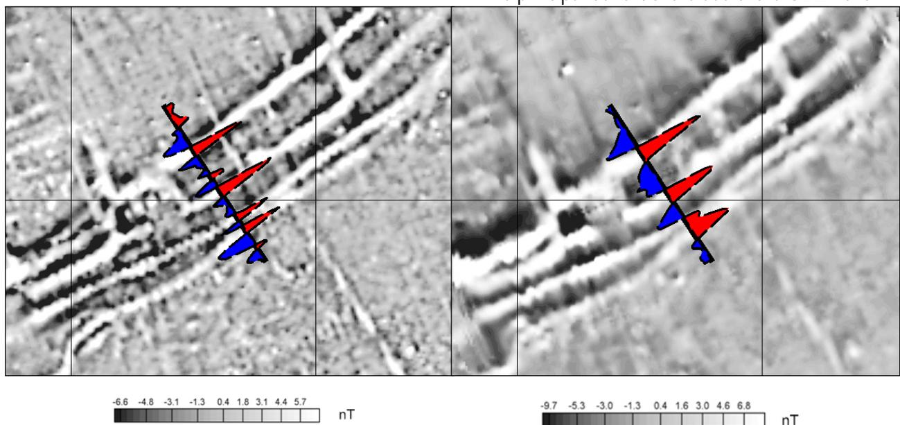
Figure 3: The magnetic profiles of each dataset over the medieval ladder settlement on a 50m grid: a) the profile of the gradiometer data; b) the profile of the total field
