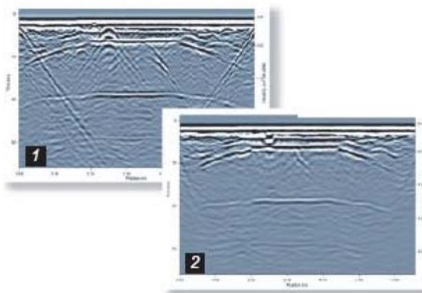
Figure 2: An initial GPR cross-section before (1) and after (2) migration processing to minimize diffraction traces and localise responses.
