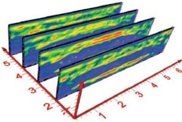
Figure 3: 3D slice view of vaulted attics cross-section created with EKKO Mapper 3 and Voxler visualization.
