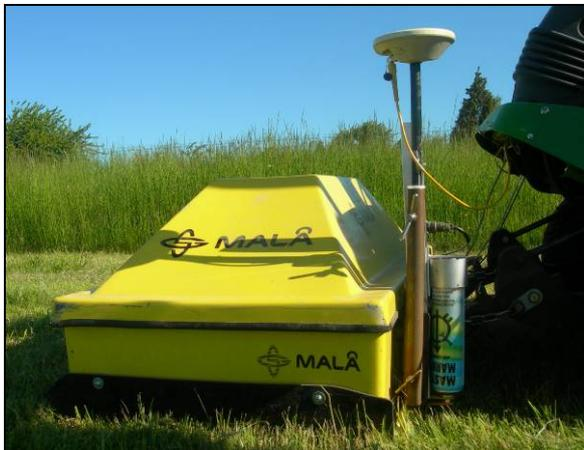
Figure 4: Antenna box with RTK-GPS antenna for positioning. The spray paint cartridge for marking on the ground is located next to the GPS-antenna shaft.
