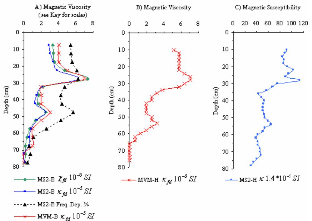
Figure 2: Borehole #1, inside House E. A) Soil samples collected at 5 cm intervals. Diamonds, squares and triangles measured on a Bartington MS2-B dual frequency sensor. Cross "X" measured on a Pulsepower Developments lab sensor. Note the different scales in the key. B) MVM1 prototype down-hole probe data collected at 2cm intervals. C) MS2-H down-hole magnetic susceptibility data collected at 2 cm intervals.
