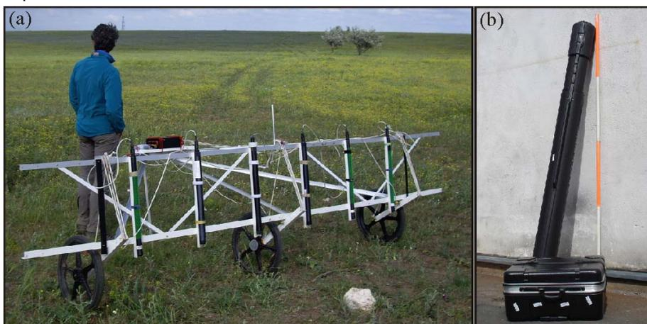
Figure 1: (a) Cart system: 4m width, set up with 6 Foerster gradiometers, sensor separation 0.5m; (b) Folded up system
