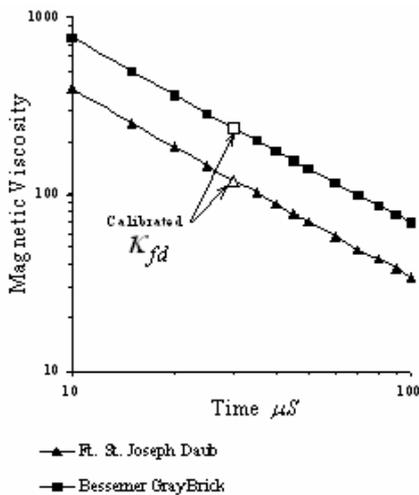
Figure 1: Log-log plot of the viscosity decay of two burnt clay samples. The first is a modern brick (Bessemer Grey from the Old Carolina Brick Co.), while the second sample is an archaeological sample of French colonial daub (late-17<sup>th</sup>-mid-18<sup>th</sup> century) from Fort St. Joseph, Michigan. The decay curves are calibrated in the time-domain to read  $\kappa_{fd}$  at 30  $\mu$ S.
