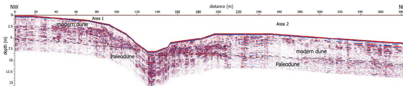
Figure 2: Radar profile with 200 MHz antenna, showing the clear reflection of the paleodune.
