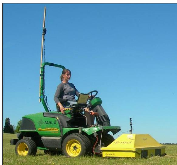
Figure 3: The Malå Imaging Radar Array mounted with hydraulic lift in front of a John Deere tractor. The yellow antenna box contains the 17 radar antennas. The prism for positioning using a robotic tachymeter can be seen next to the antenna box.
