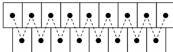
Figure 2: Sketch MIRA antenna arrangement. Dotted lines indicate transmitter and receiver antenna combinations.
