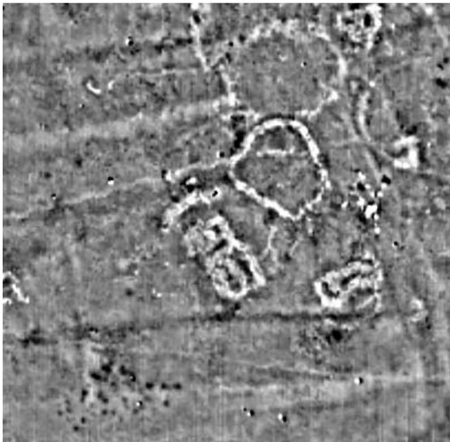
Figure 2: Geomagnetic results; size: 100m x 100m; line separation 0.5m; inline sample separation 0.05m; dynamic range  $\pm 6nT$ .
