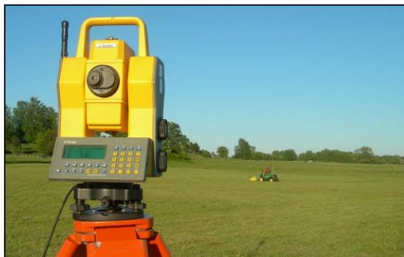
Figure 5: Robotic tachymeter (total station) with the MIRA system visible in the background.
