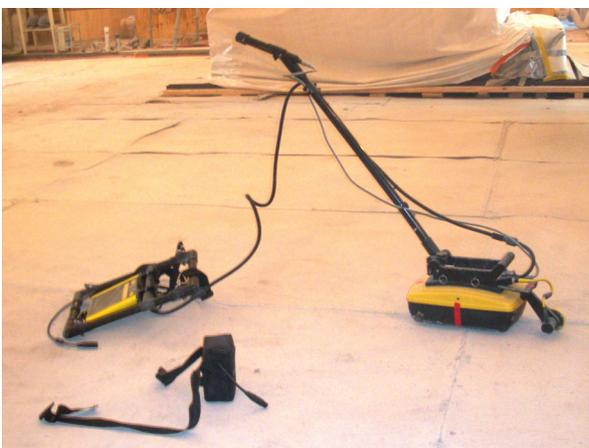
Figure 1: Hand-tow GPR system with 500 MHz antenna and attached small odometer wheel for in-line positioning. An adjustable handle bar with rigid mounting permits good control over antenna movement.
