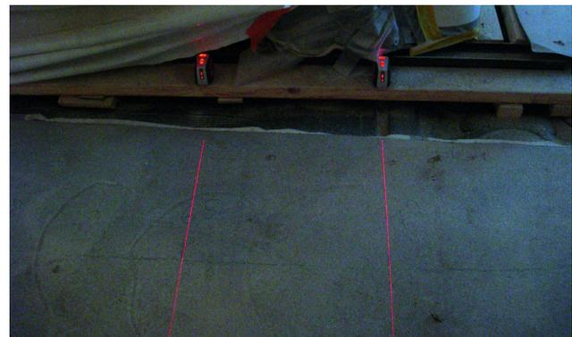
Figure 2: Two laser levels spaced at 50 cm distance emitting parallel lines of light clearly visible on the floor.
