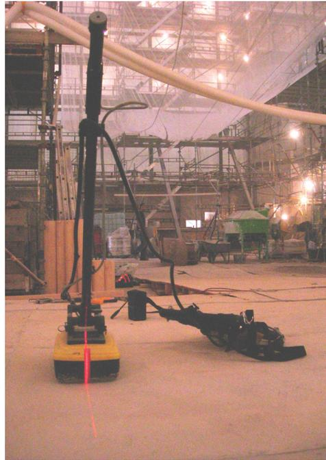
Figure 4: Laser beam focused on the centre of the GPR antenna while pulling the system towards the laser level.
