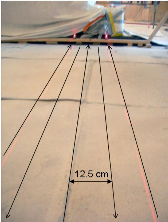
Figure 3: Illustration of the survey scheme using a spacing of 50 cm between the two laser levels and a cross-line GPR profile spacing of 12.5 cm.
