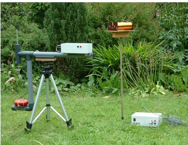
Figure 1: The prototype instrument, comprising a portable single channel magnetometer, and associated static reference instrument.
