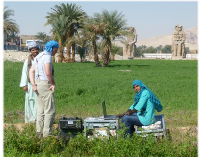
*Figure 1 ERT survey being conducted to the east of the Colossi of Memnon, West Bank, Thebes (photo: Angus Graham)*
