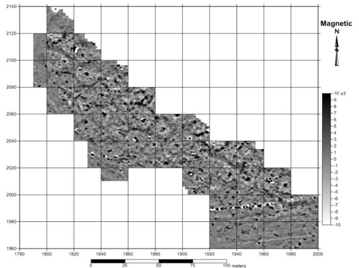
**Figure 5. Image plot of the 2012 magnetic data.**
