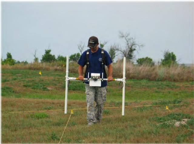
**Figure 3. Collecting magnetic data with the dual fluxgate gradiometer.**
