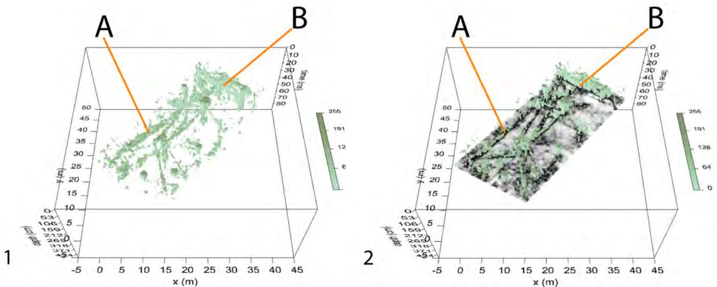
**Figure 4: Volumetric visualisation the GPR survey results at Sant'Ivo alla sapienza: 1, Isosurface rendered image using amplitude values above 99.9% of maximum amplitudes; 2, Isosurface image combined with horizontal time-slice of an approximate depth of 10.7ns or 56.72cm.**
