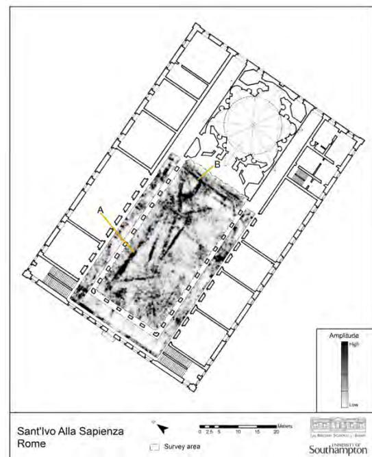
**Figure 2: GPR survey results (depth approximation 15-17ns:79-90cm). Two linear anomalies (A and B) have been identified as potentially having an archaeological significance.**
