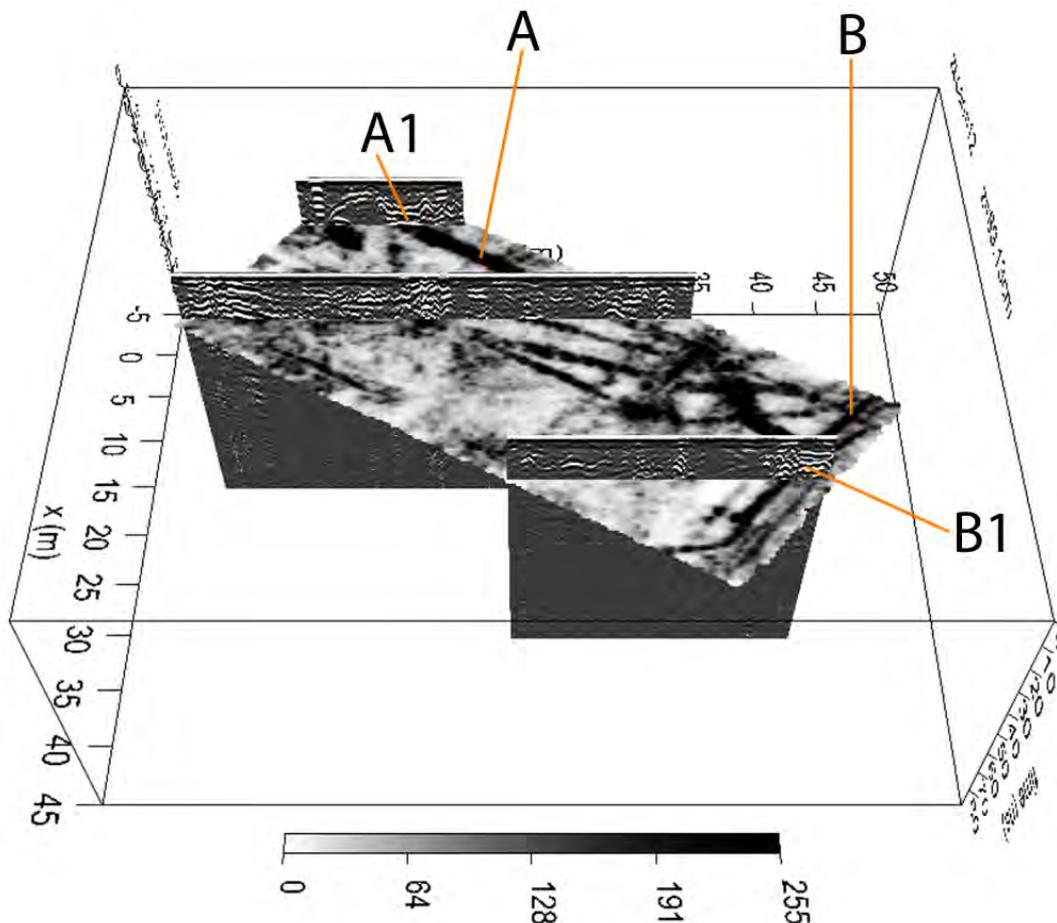
**Figure 3: Visualisation showing unprocessed radargrams (traverses 20, 60 and 120) and a processed time-slice with a depth approximation of 16.82ns or 89.13cm. Features labelled 'A and B' their corresponding hyperbole marked 'A1 and B1' are suggested to indicate the presence of structural remains.**
