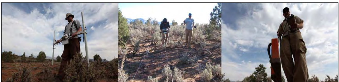
Figure 2 Bartington 601 magnetometer, Geoscan RM15 resistivity meter(survey collaboration with Mona Charles, Fort Lewis College), Geonics EM38B conductivity meter.
