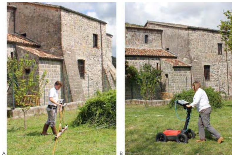
Figure 2: Data collection during the: A, resistance survey; and B, GPR survey
