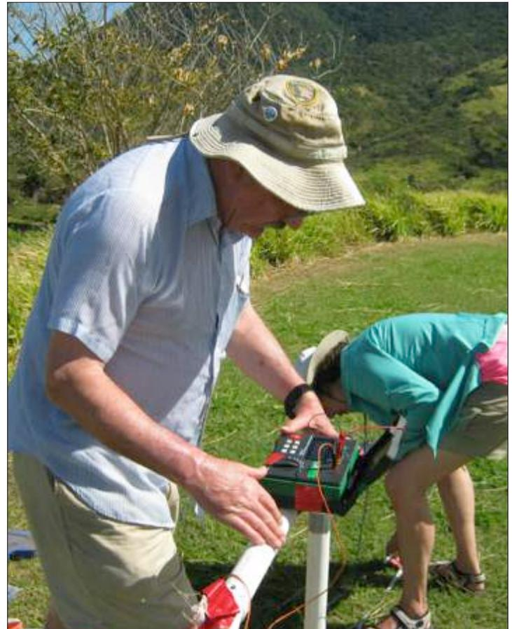
**Figure 1** Photo of the author operating the DY4300 resistivity meter mounted on the PVC pipe frame.
