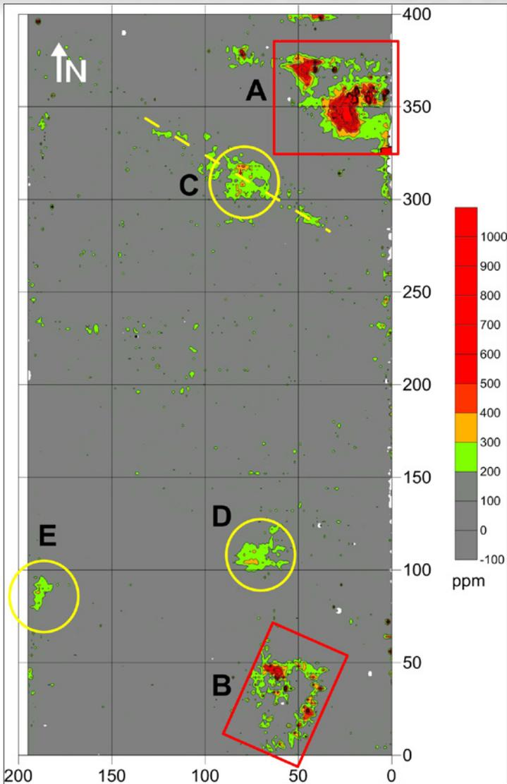
**Figure 2** In-phase results ('magnetic susceptibility') revealing two intensely anomalous areas (A and B), as well as three other areas of interest (C, D, and E). Anomaly C may be anthropogenic, but it may also have a geological origin (dotted line).
