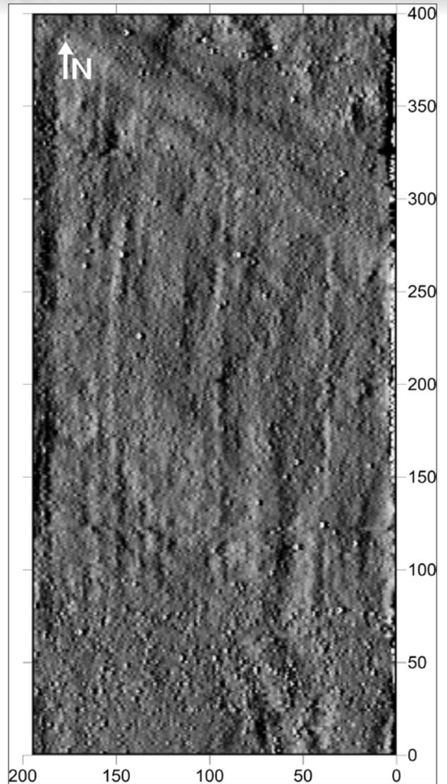
**Figure 3** Conductivity data plotted as a shaded relief map. Several linear field boundaries, which do not find expression in the susceptibility data, are readily apparent.
