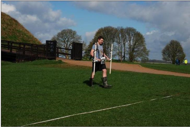
**Figure 2 (top left)** Magnetometer survey using a Bartington Instruments Grad 601-2 fluxgate gradiometer in the outer bailey of Old Sarum.
