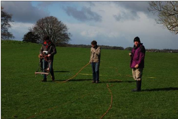
Noggin Plus system with 500Mhz antenna and Smartcart in the outer bailey. Data were collected along traverses spaced 0.5m apart. Data were processed using GPR Slice software.
