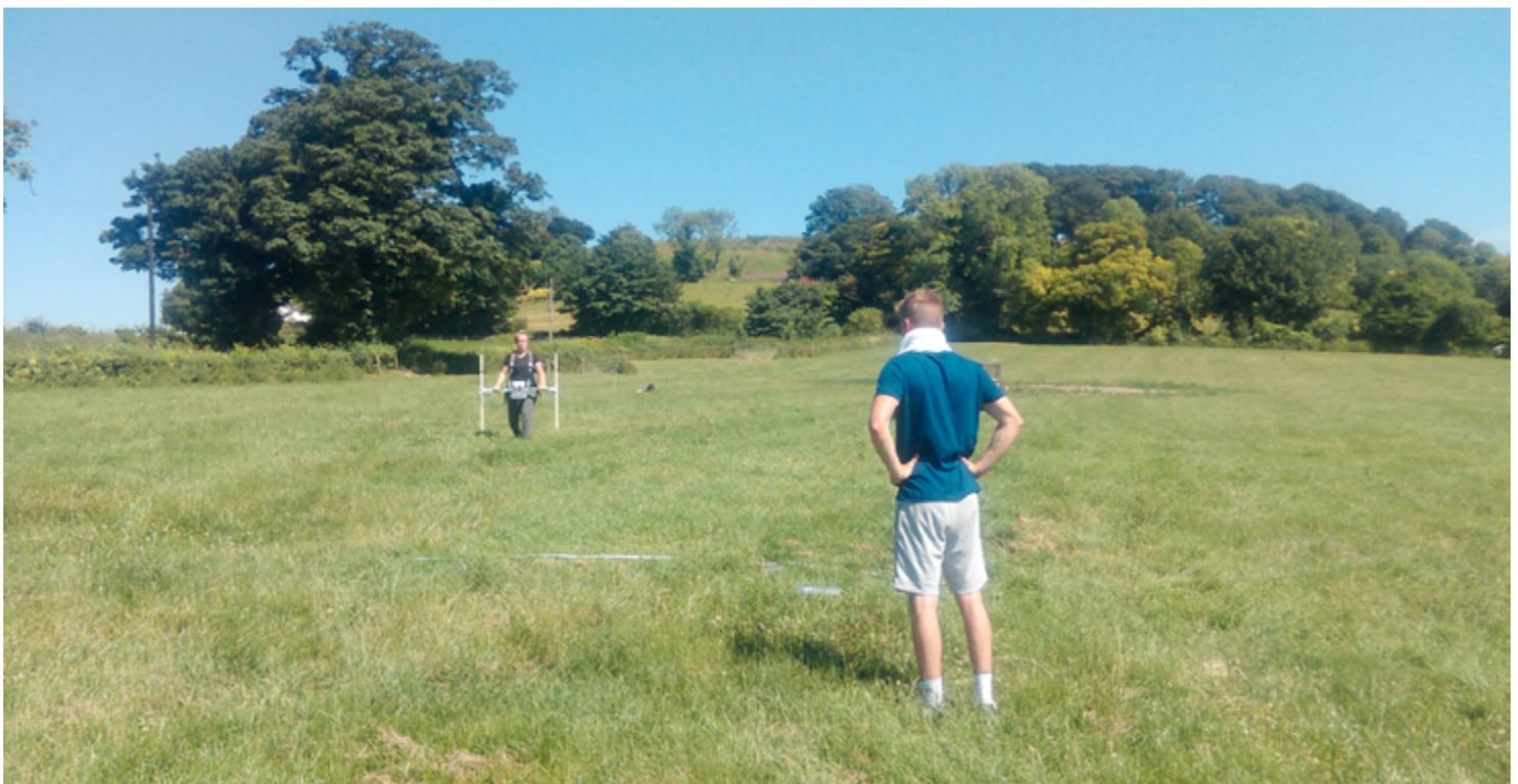
**Figure 3** Magnetometer survey being conducted using a Bartington Instruments Grad 601-2 fluxgate gradiometer.
