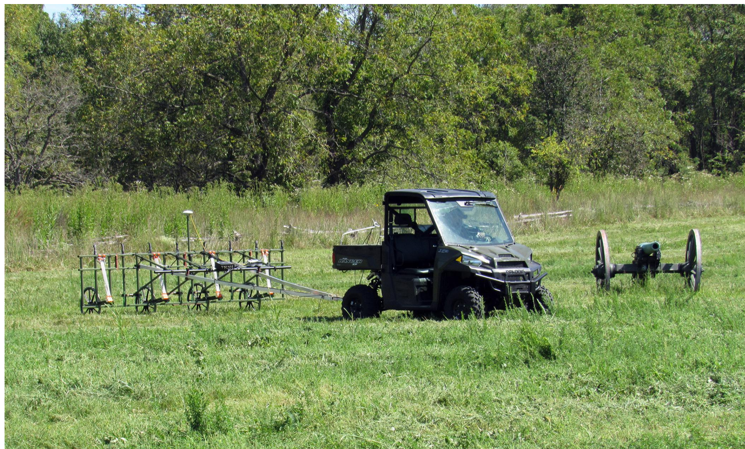
Figure 1: Fluxgate gradiometer survey performed at Pea Ridge National Military Park with an 8-channel SENSYS MAGNETO MX V3.
