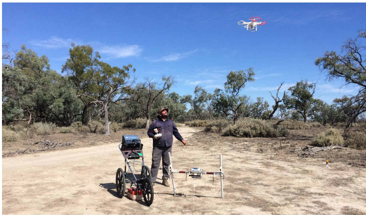
Figure 4: Ian Moffat with the GSSI Sir3000 GPR with 400 MHz antenna, Bartington Grad 601 magnetometer and DJI Phantom 3 Professional used for this survey.
