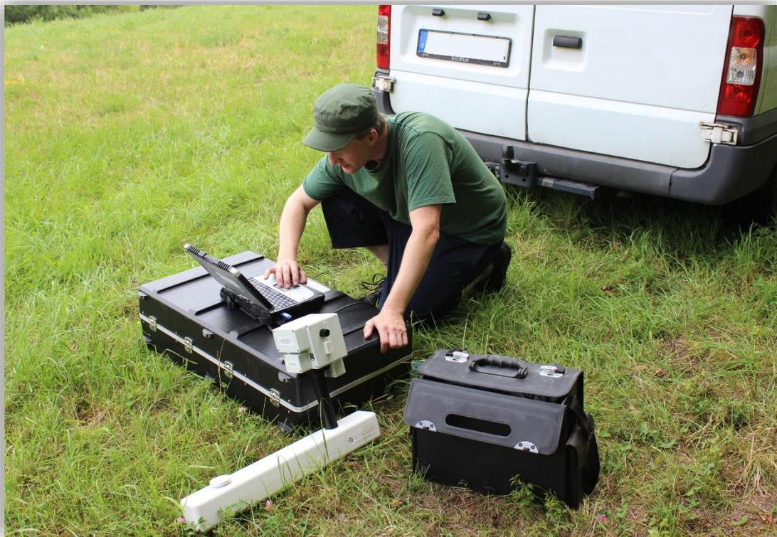
19. **Data Dumping:** Data transfer from a Geoscan FM256 in the field. – most members will have done this at some point – Benny Rieger
