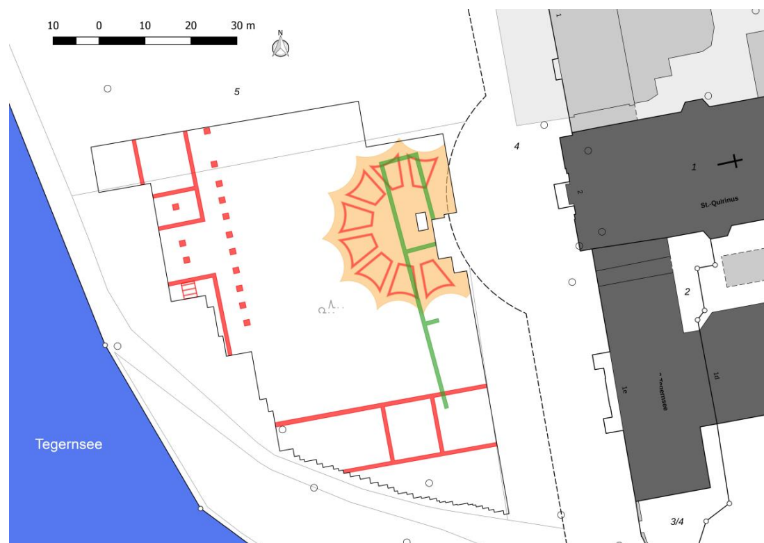
Figure 4: Digital interpretation plan of the GPR survey. Colour coding: red = Baroque walls of monastery, green = pre-Baroque building phase, orange = garden architecture, black = survey grid (© BLfD, 2020).
