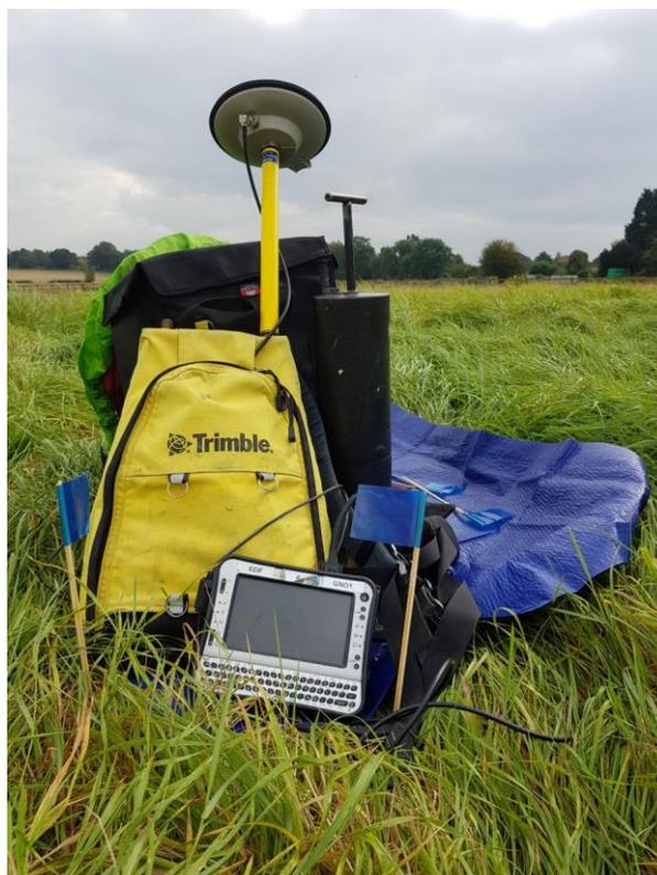
*Figure 1: The Groundhog Fusion System gamma-ray detector as trialled at Roman Silchester*
