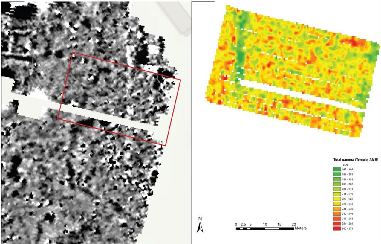
*Figure 2: Geophysical survey image (left) and gamma-ray spectrometer survey image (right) at the Temple site in Silchester. The boundary wall (Temenos wall) is visible as a green shape, indicating low radiation relative to the surrounding soil. This could indicate that the materials used to build the wall were imported from a different location and could have been made from a material with lower concentrations of naturally occurring radioactivity, such as sandstone*
