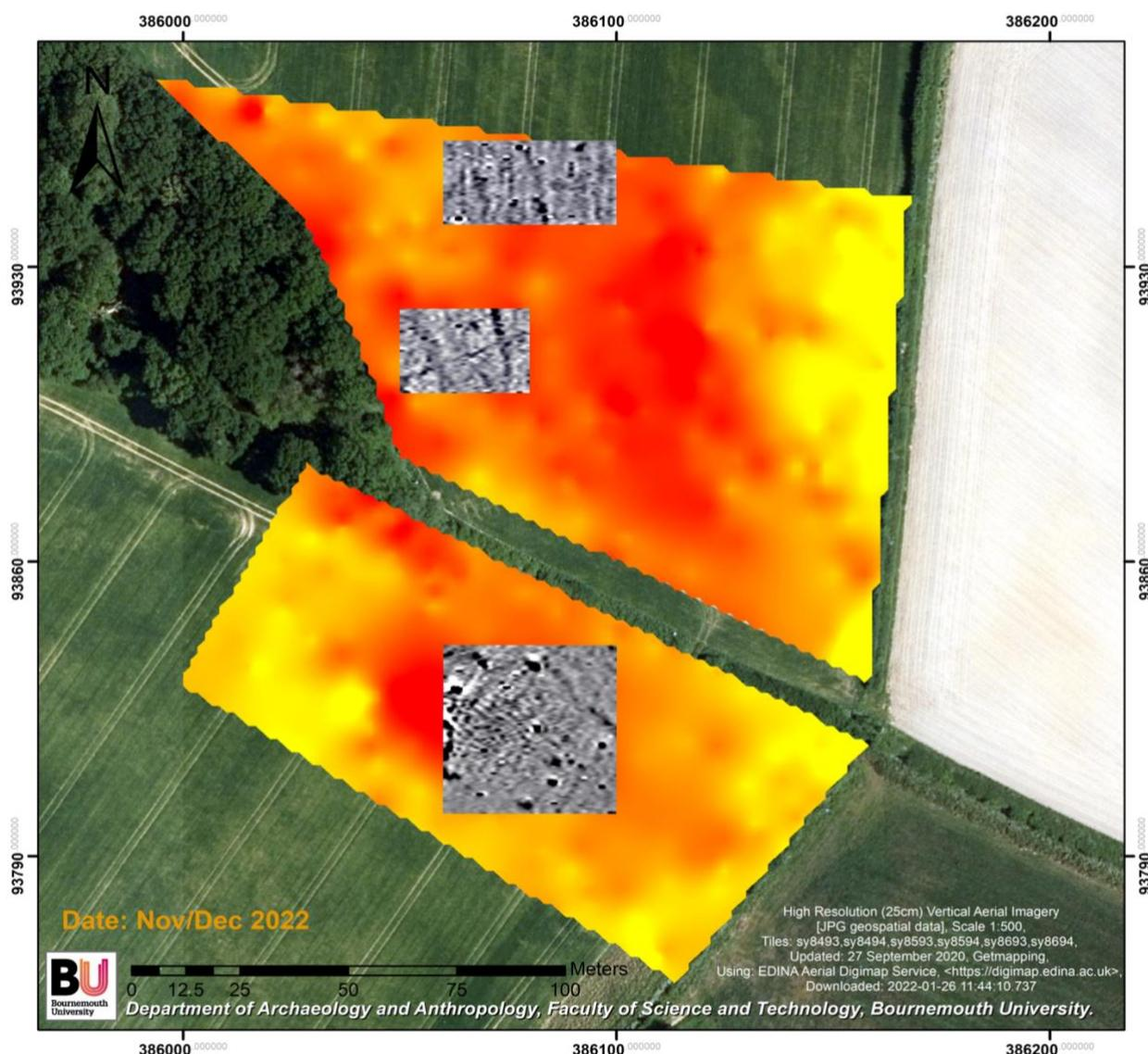
*Figure 2: In areas that have been allowed to naturally regenerate it is not possible to conduct extensive areas of gradiometry and so topsoil magnetic susceptibility survey has been used as the primary prospection technique. In this case it has followed up by restricted areas of gradiometry to confirm the presence and some idea of the nature of an archaeological site. Bartington MS3 + MS2D coil with a c. 7 m (uncorrected HH GPS) survey interval. Log scaled: high susceptibility = red.*
