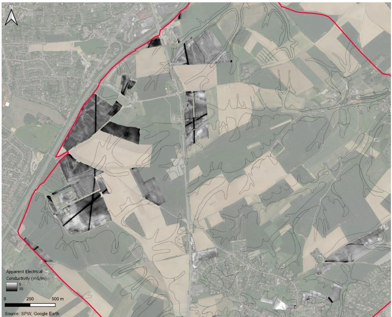
*Figure 5: Overview of apparent electrical conductivity (1 m horizontal coplanar coil pair) for entire surveyed area. Note especially the linear resistive zones correlating well with colluvial deposits (shown by the overlaid black outlines from mid-20th century soil surveys). The red outline indicates the protected battlefield zone (as shown in Figure 1).*
