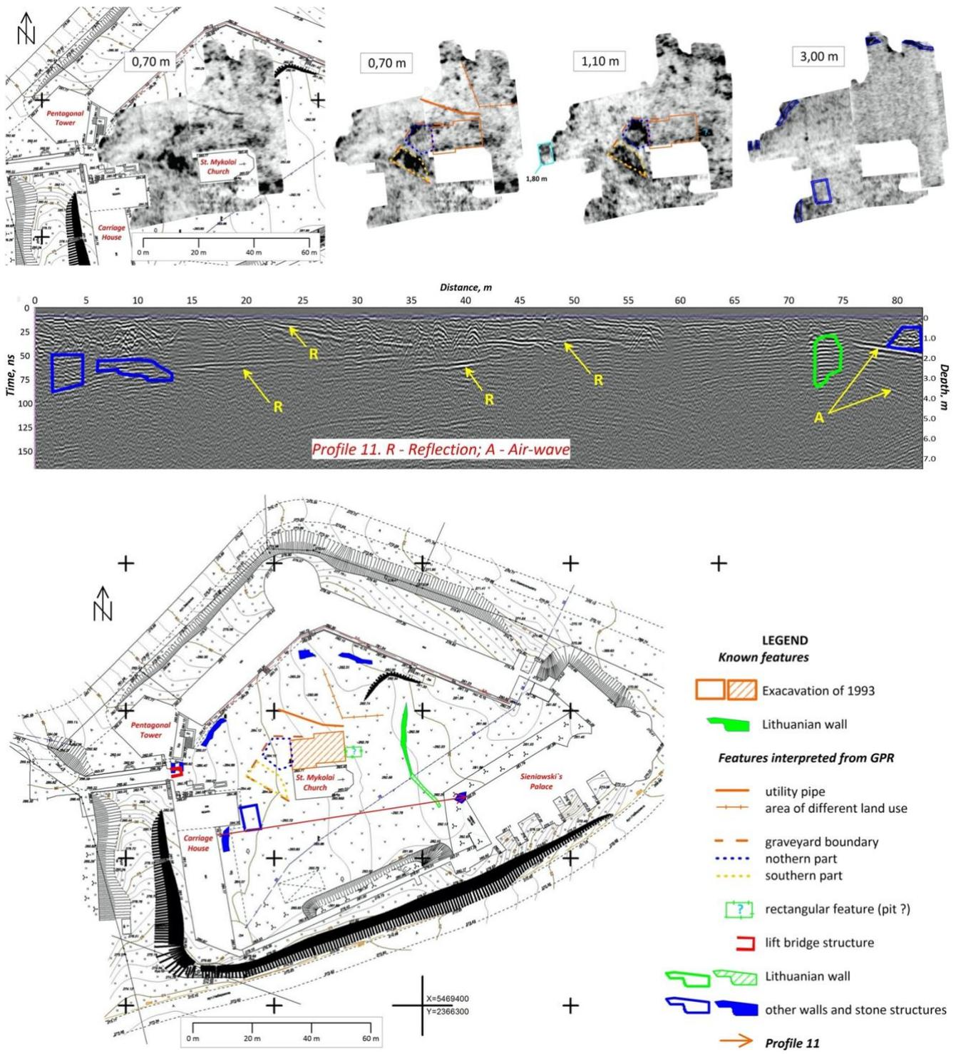
Figure 1: GPR survey results from the courtyard of Medzhybizh Fortress. Top: selected time slices and radargram with interpretation. Bottom: recognized structures overlaid on topographic plan.
