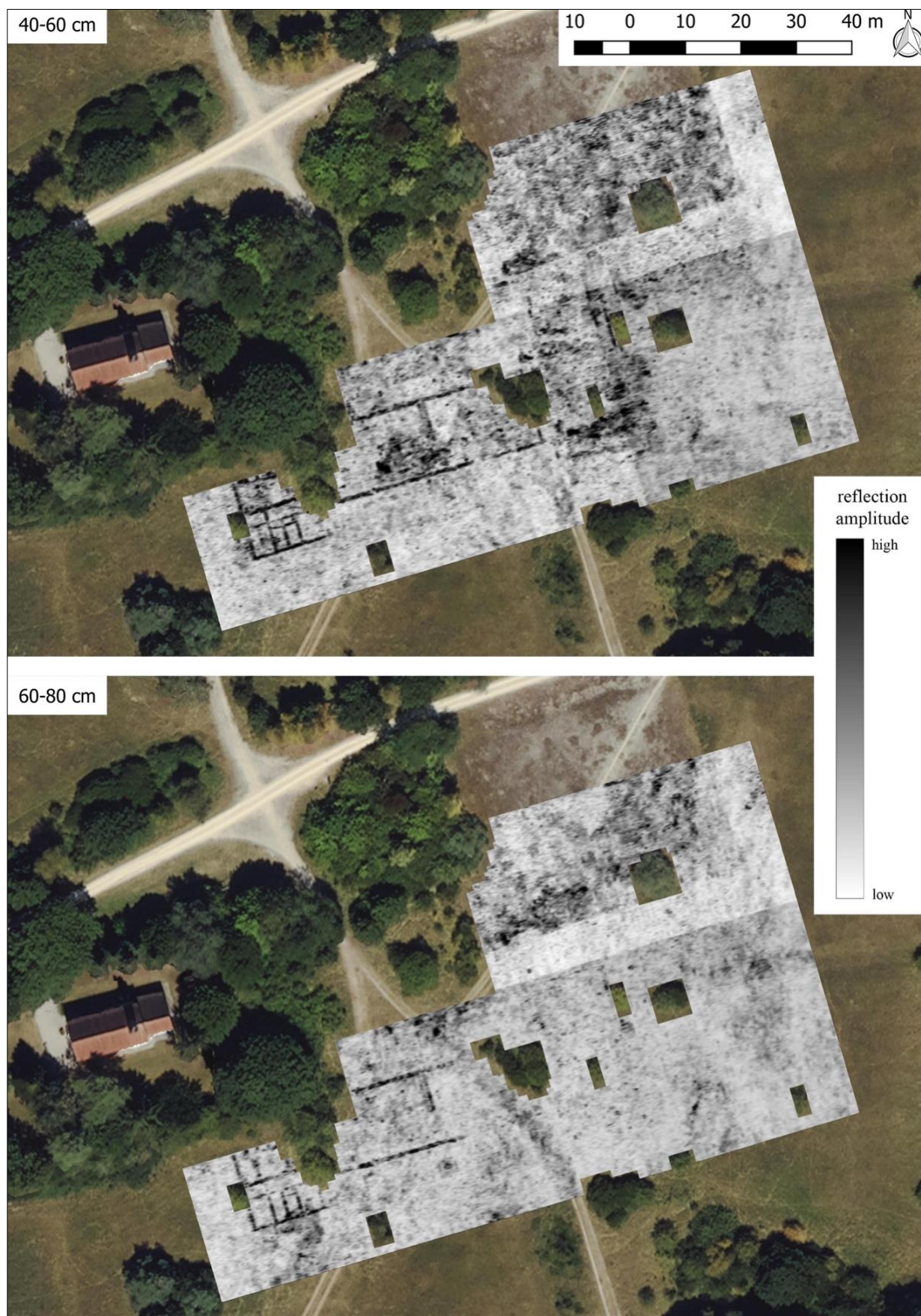
Figure 2: Selection of depth slices in the relevant range of 40-80 cm below the modern surface. GSSI SIR-4000 with 400 MHz-antenna, sample interval: 6 x 25 cm. Project-No. Mal23rad.
