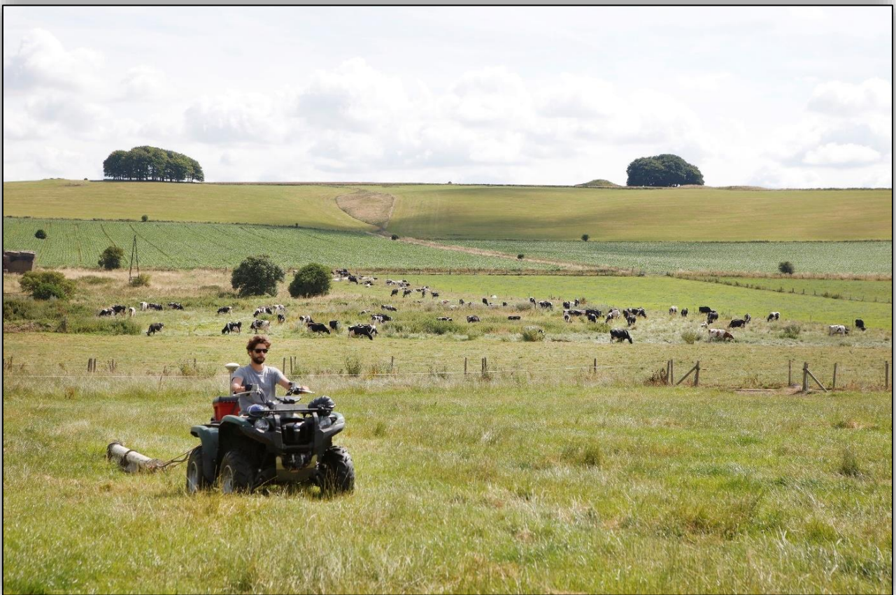
Philippe De Smedt carrying out a motorized EMI survey in short sleeves. Picture by Layla Aerts, provided by Jeroen Verhegge.
