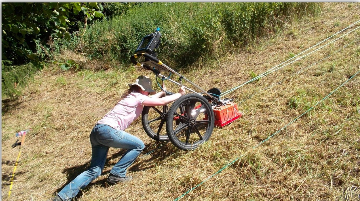
Crazy GPR survey of a 45° steep hill in search of a possible Roman theatre in Southern Bavaria. The standard GPR equipment was modified to fit the special requirements of the survey area. The kit was pulled with a rope and a tackle from above. Picture and description by Roland Linck.
